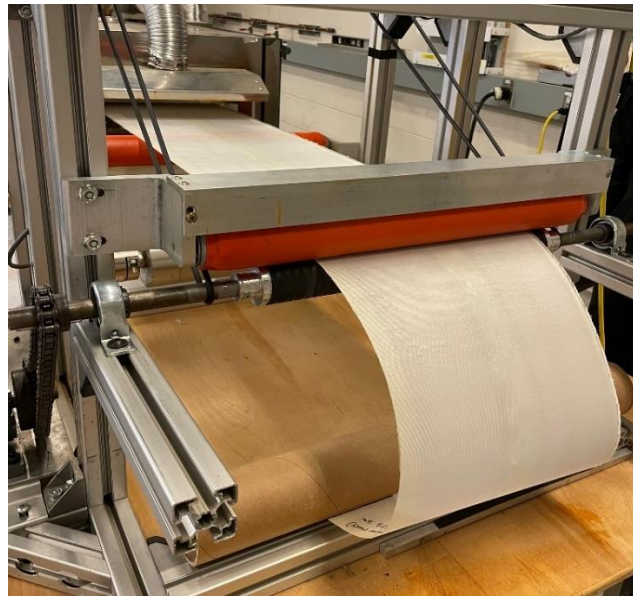
Figure 4. Conveying rollers installed on the take-up section of treater.
