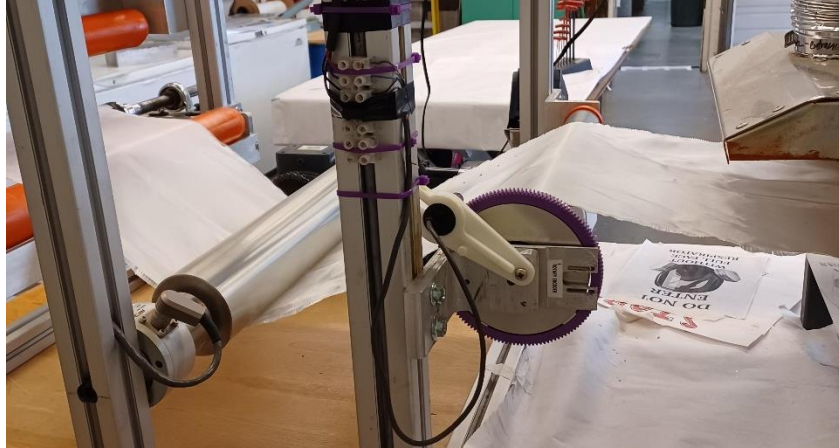
Figure 11. Speed sensing roller and tension roller repositioned at take-up section
