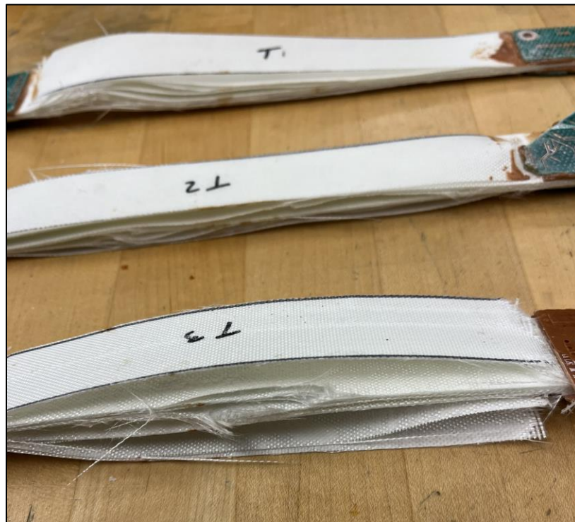
Figure 10: 3 examples of the fiberglass tensile bars after fracture.
