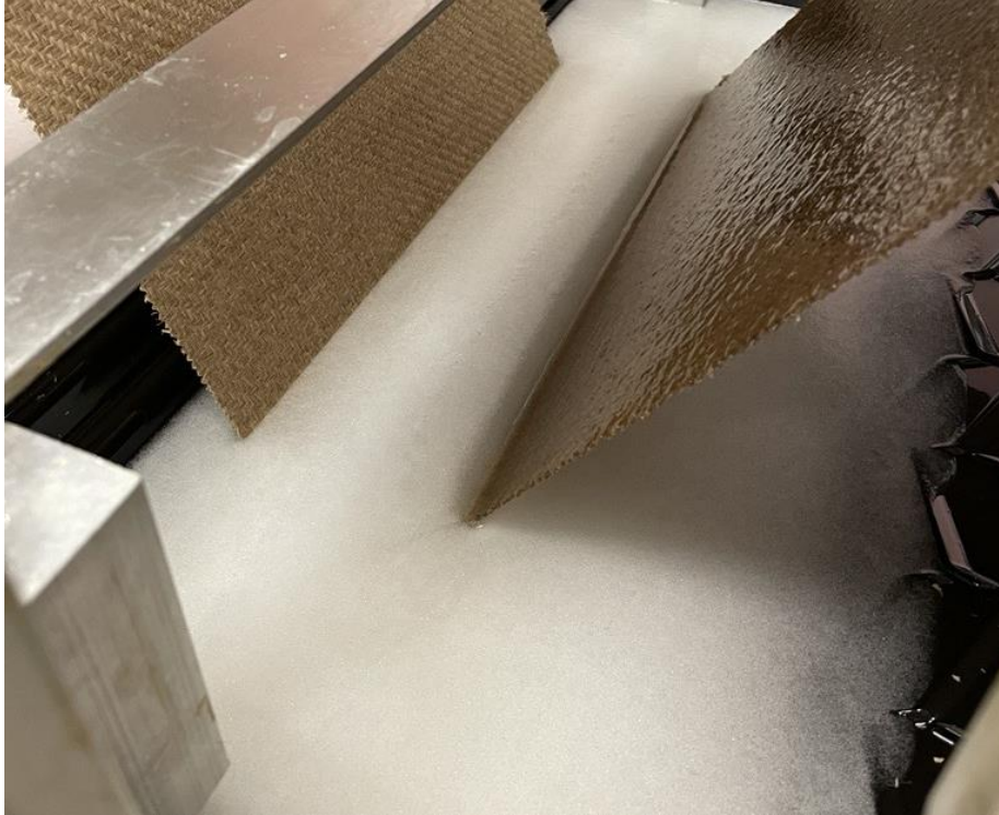
Figure 19. White foam present underneath the pinch rollers in the resin bath.
