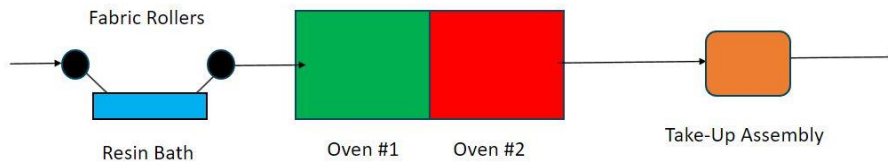
Figure 2. Simple 2D diagram of Treater Configuration for Thermosets.
