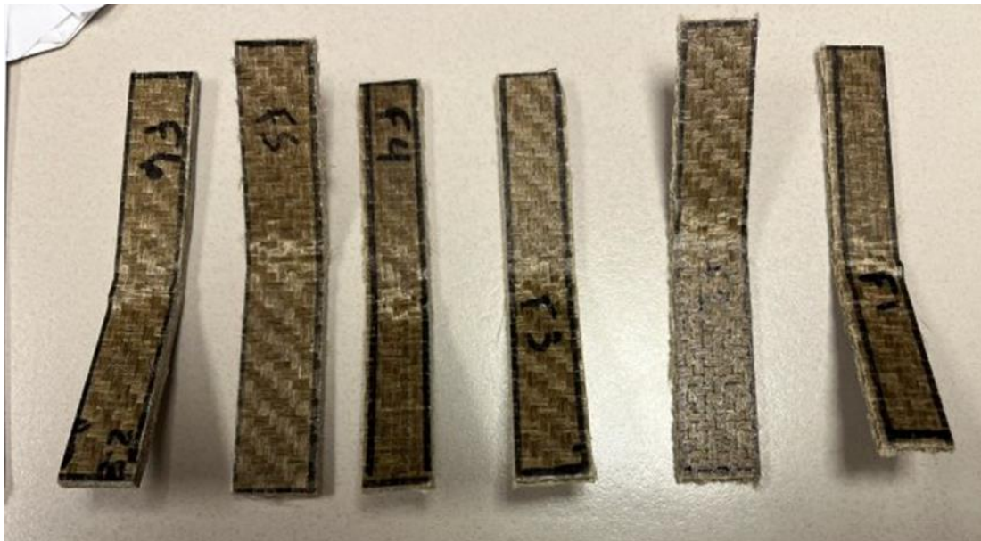
Figure 15: 6 Flax flexural bars after testing.
