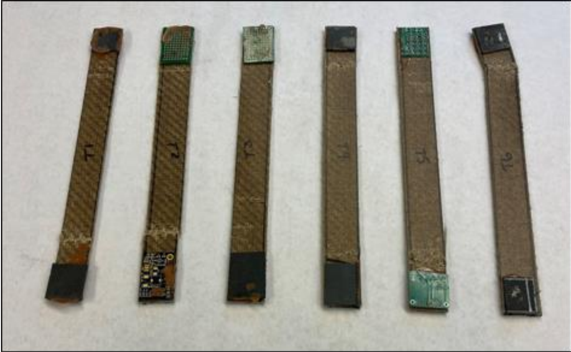
Figure 9: 6 Tensile bars broken, featuring the same failure mode near the grips.
