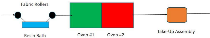
Figure 3: Simple 2D diagram of Current Treater Configuration
