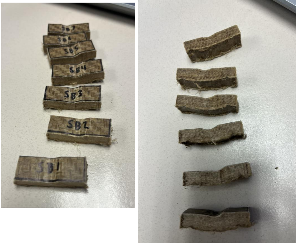
Figure 13: Flax short beam shear failures, top (left) and side (right) views.
