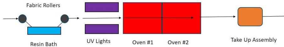
Figure 13: WWU Lab-Scale Treater, Modification Option 2
