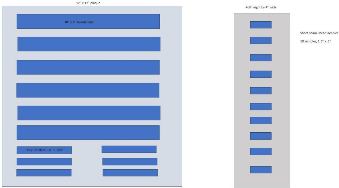
Figure 5: Layout of composite coupons
