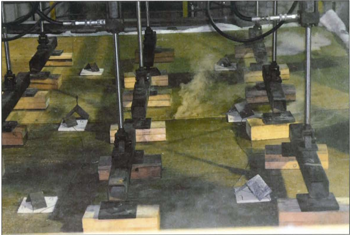
Figure C-5. Smoke from Seam of Serial No. 4001a Floor Assembly 18 min into Test.
