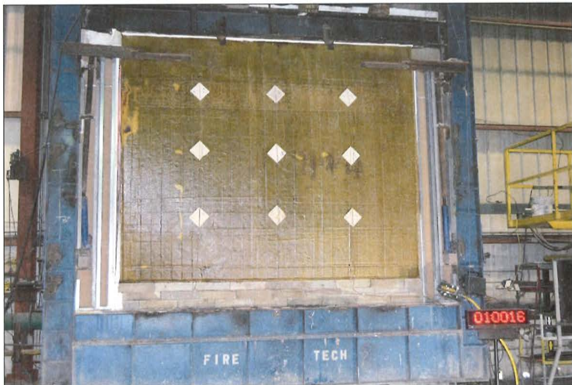
Figure C-8. Unexposed Side of Serial No. 4001b Wall Assembly 1 h into Test.
