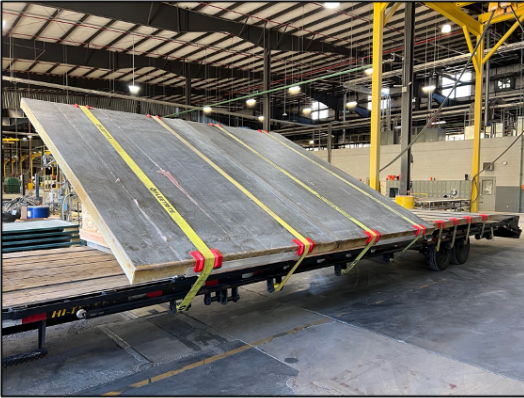
12'-8" x 15'-8" floor panel. Note floor panel was molded in two pieces and adhesively-bonded in a tongue/groove joint
