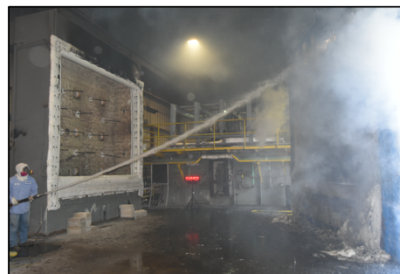
60 second fire hose spray
