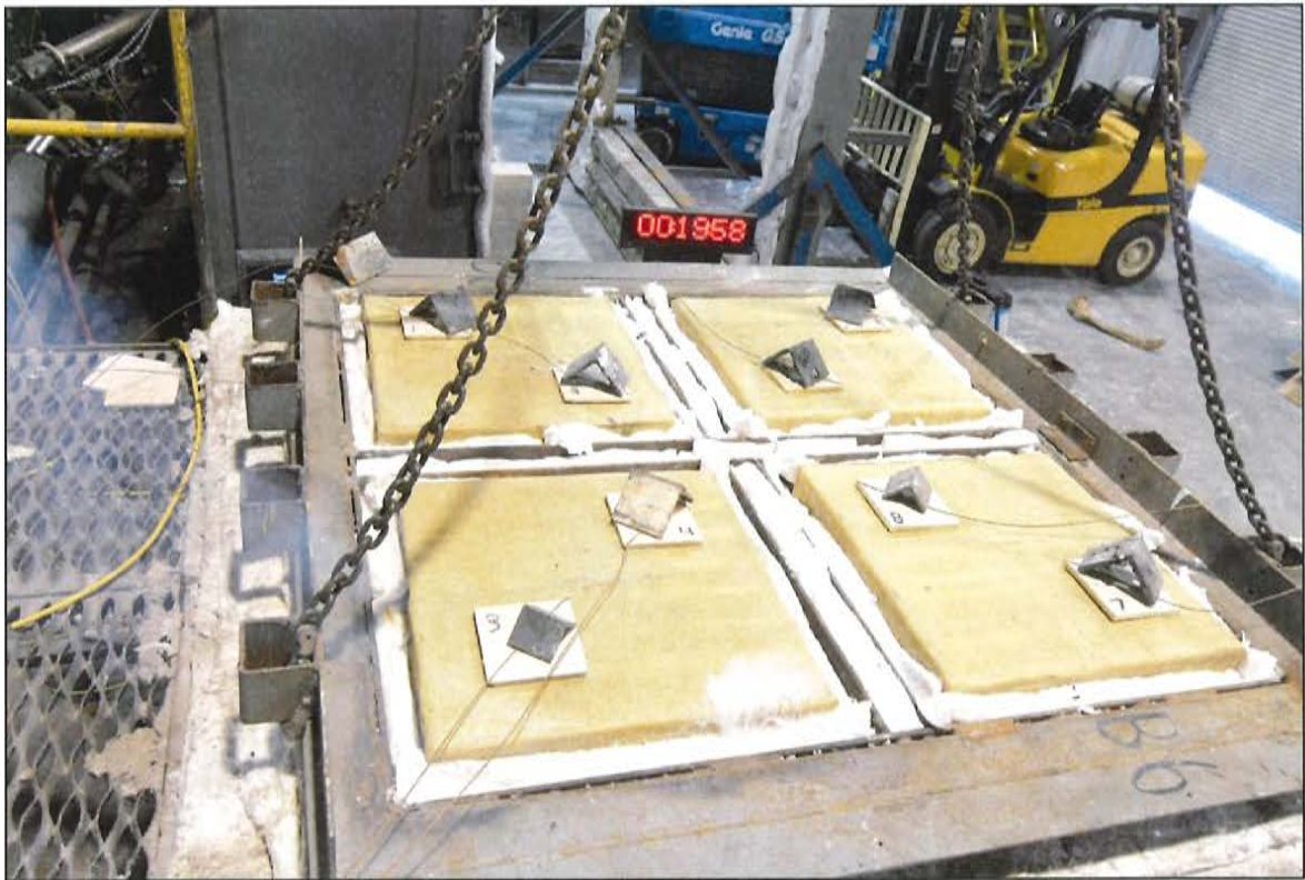
Figure B-3. Unexposed Side of Orenco Systems Samples at 20 min into the Test.
