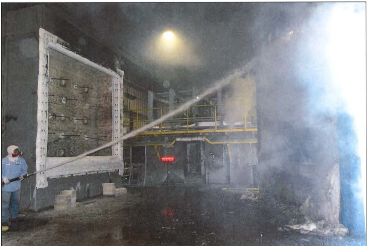
Figure C-10. Hose Stream Test in Progress.
