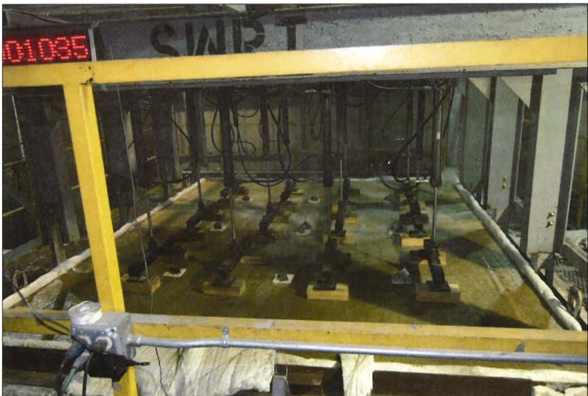
Figure C-4. Unexposed Side of Serial No. 4001a Floor Assembly 10 min into Test.
