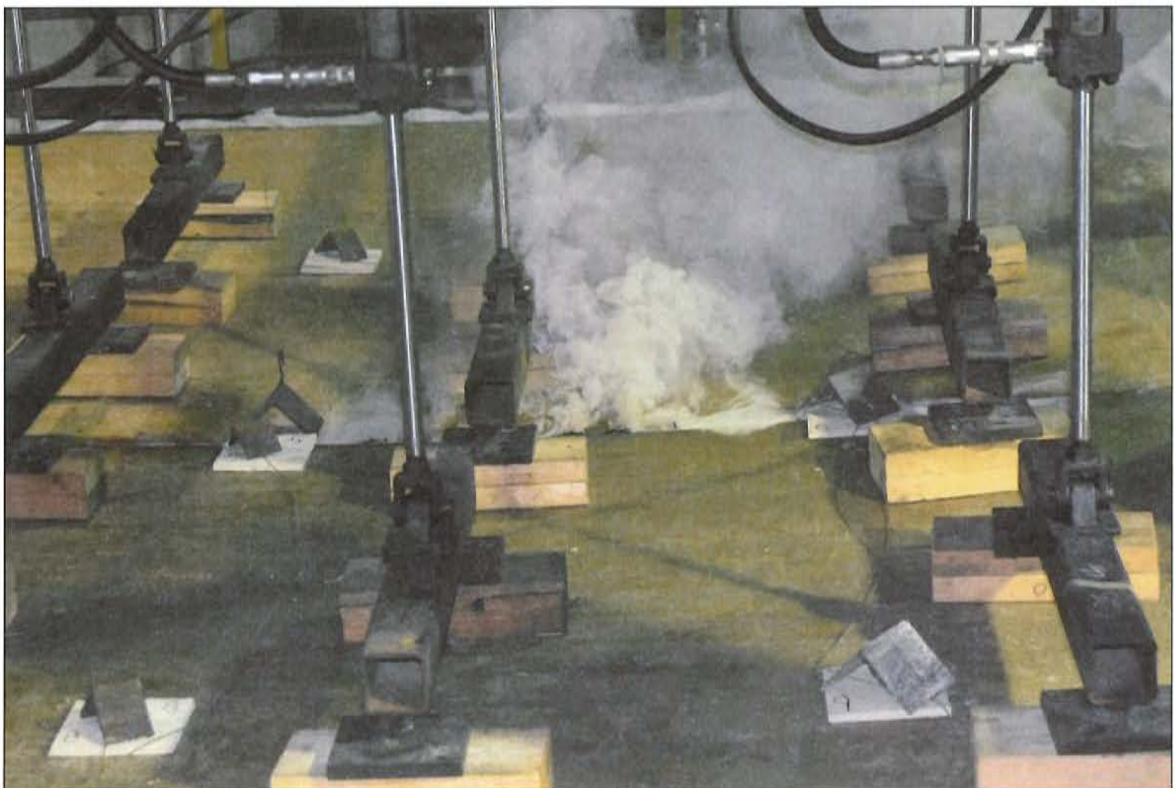
Figure C-8. Smoke from Seam on the Unexposed Side 47 min into Test.
