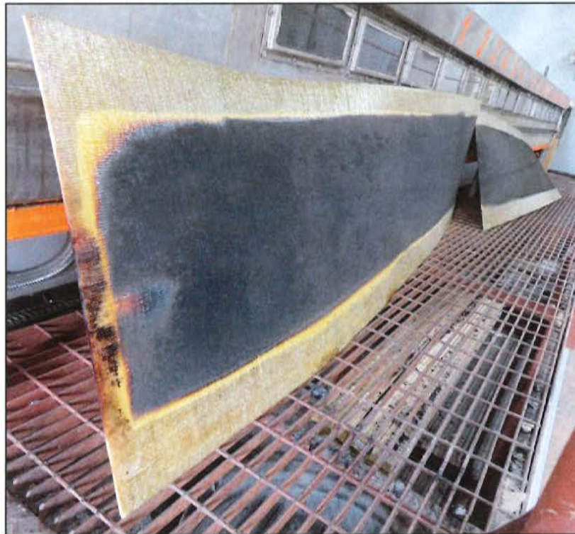
Figure B-2. Exposed side of the material after fire exposure.
