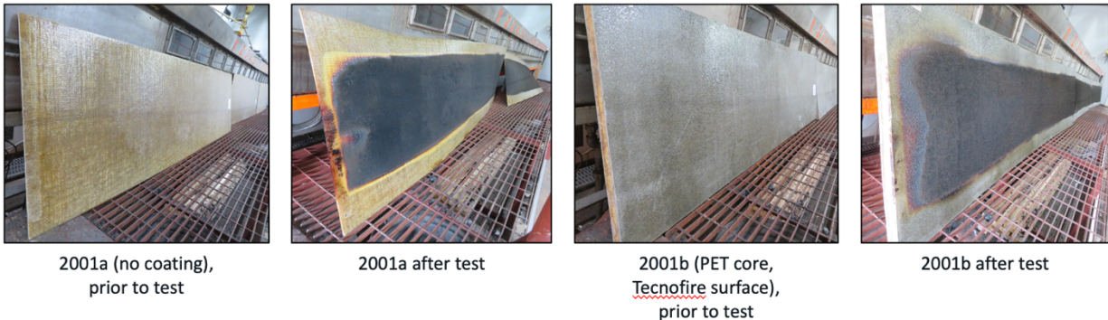
Figure 6. E84 test photos
