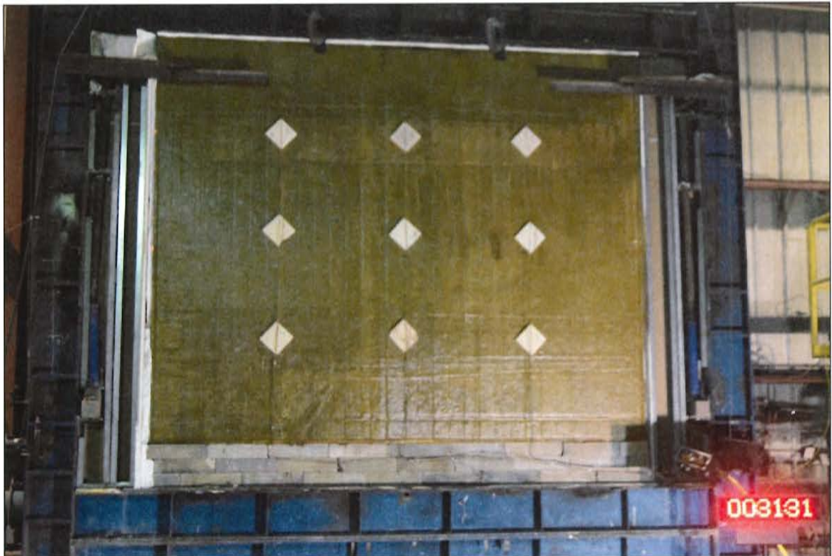
Figure C-6. Unexposed Side of Serial No. 4001b Wall Assembly 31 min into Test.
