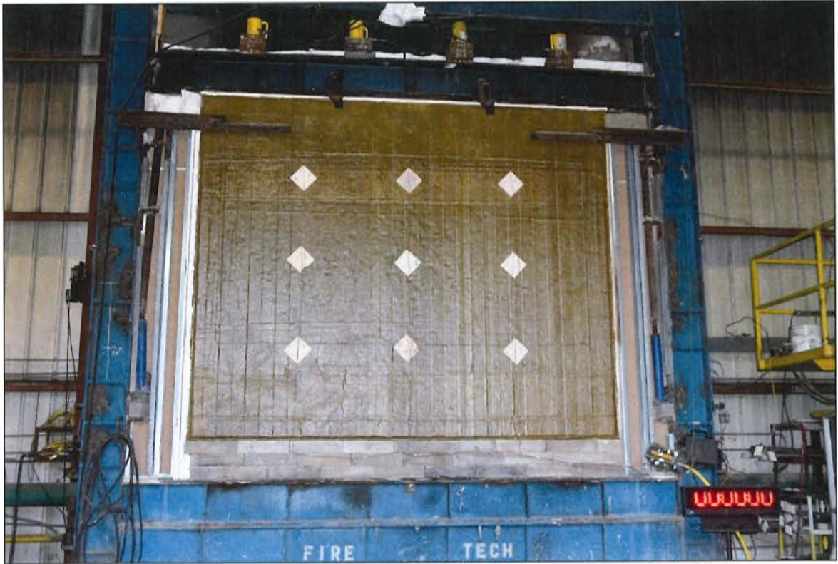
Figure C-3. Unexposed Side of Serial No. 4001b Wall Assembly prior to Testing.
