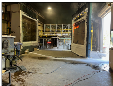
Panel frame removed from furnace
