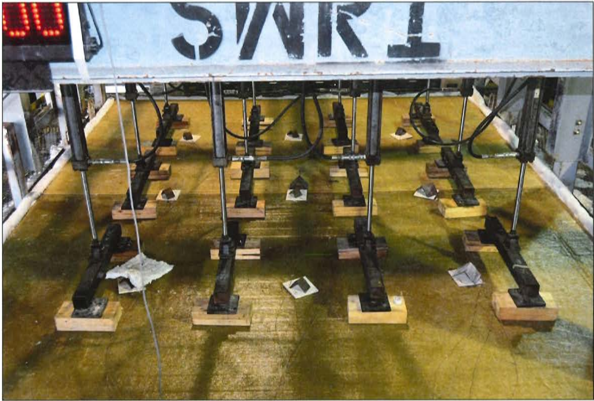
Figure C-3. Unexposed Side of Serial No. 4001a Floor Assembly prior to Testing.
