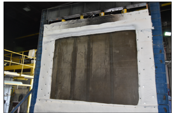
Test side prior to installation against furnace
