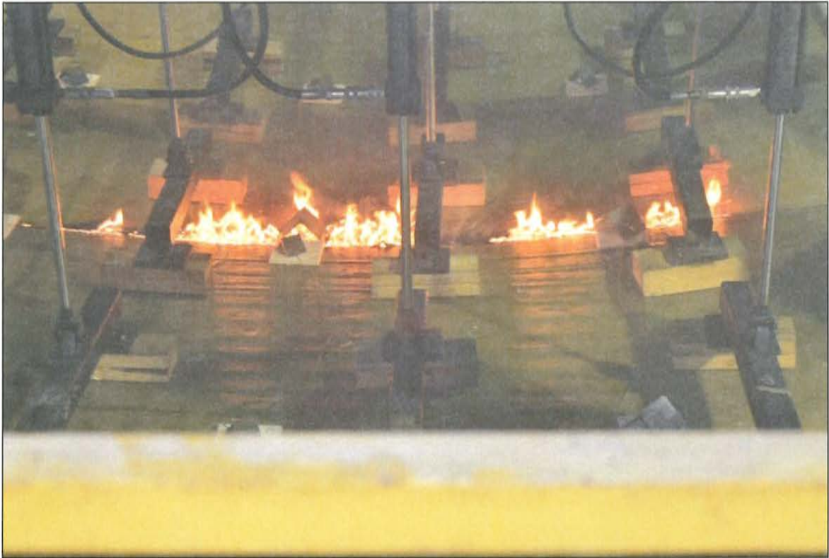
Figure C-9. Flames from Seam of Serial No. 4001a Floor Assembly 56 min into Test.
