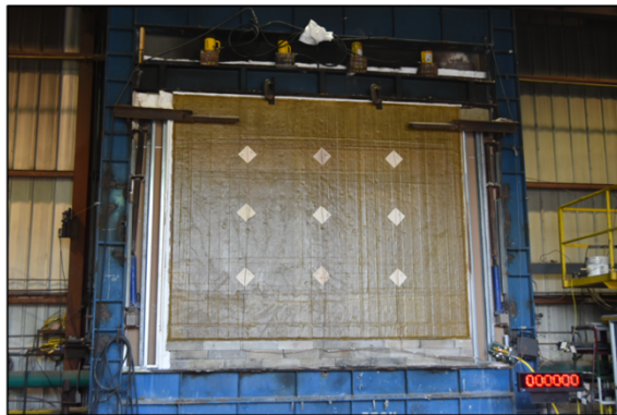
12 ft wide x 9 ft tall wall panel ready to start test
