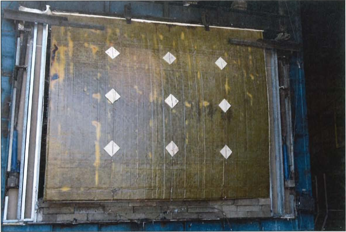
Figure C-11. Unexposed Side of Serial No. 4001b Wall Assembly after Hose Stream Test.
