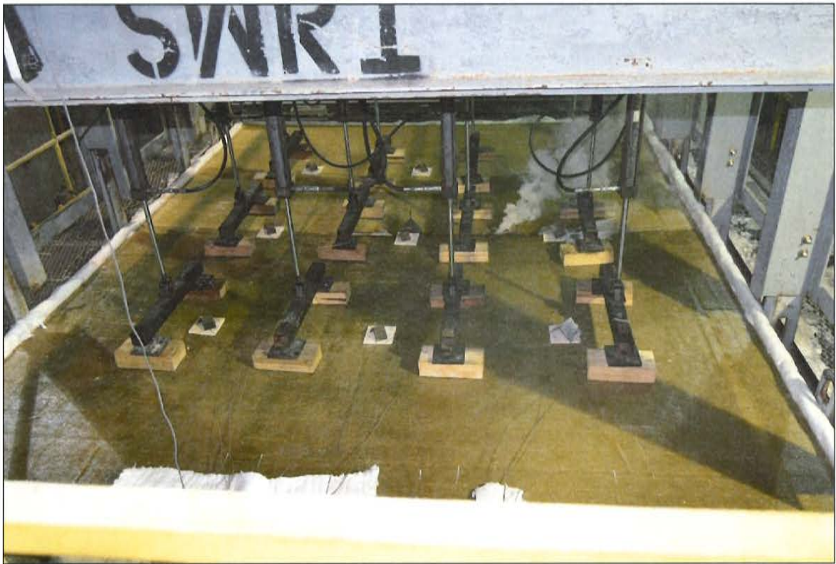
Figure C-7. Left Edge of Serial No. 4001a Floor Assembly 40 min into Test.
