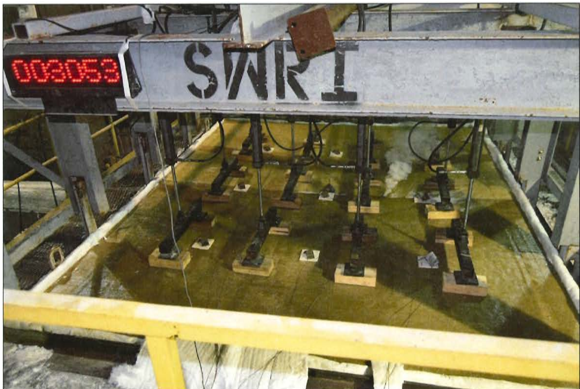
Figure C-6. Unexposed Side of Serial No. 4001a Floor Assembly 30 min into Test.
