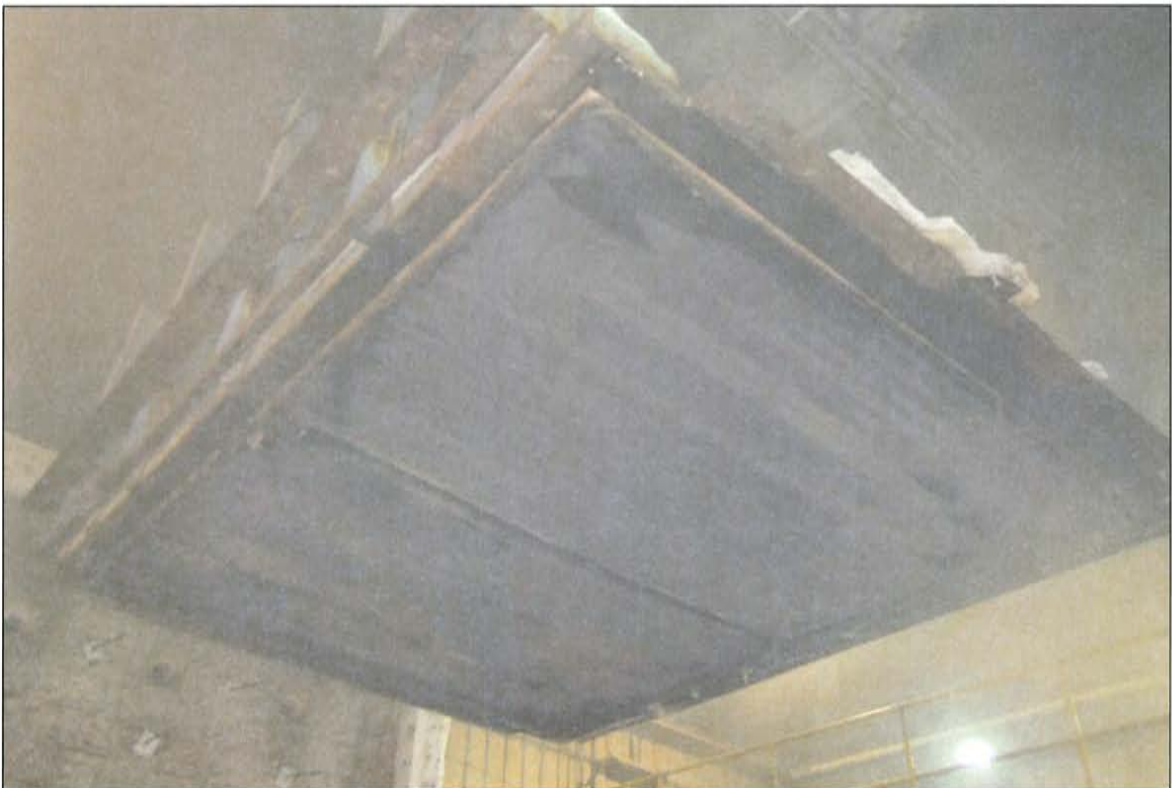
Figure C-10. Exposed Side of Serial No. 4001a Floor Assembly during Removal from Furnace.
