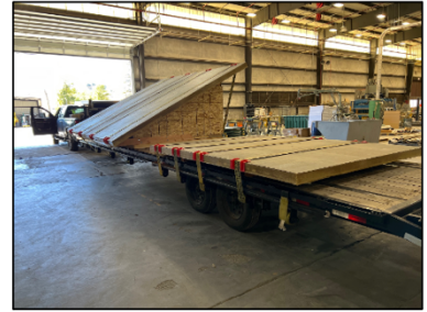
Wall & floor panels shipping to SwRI
