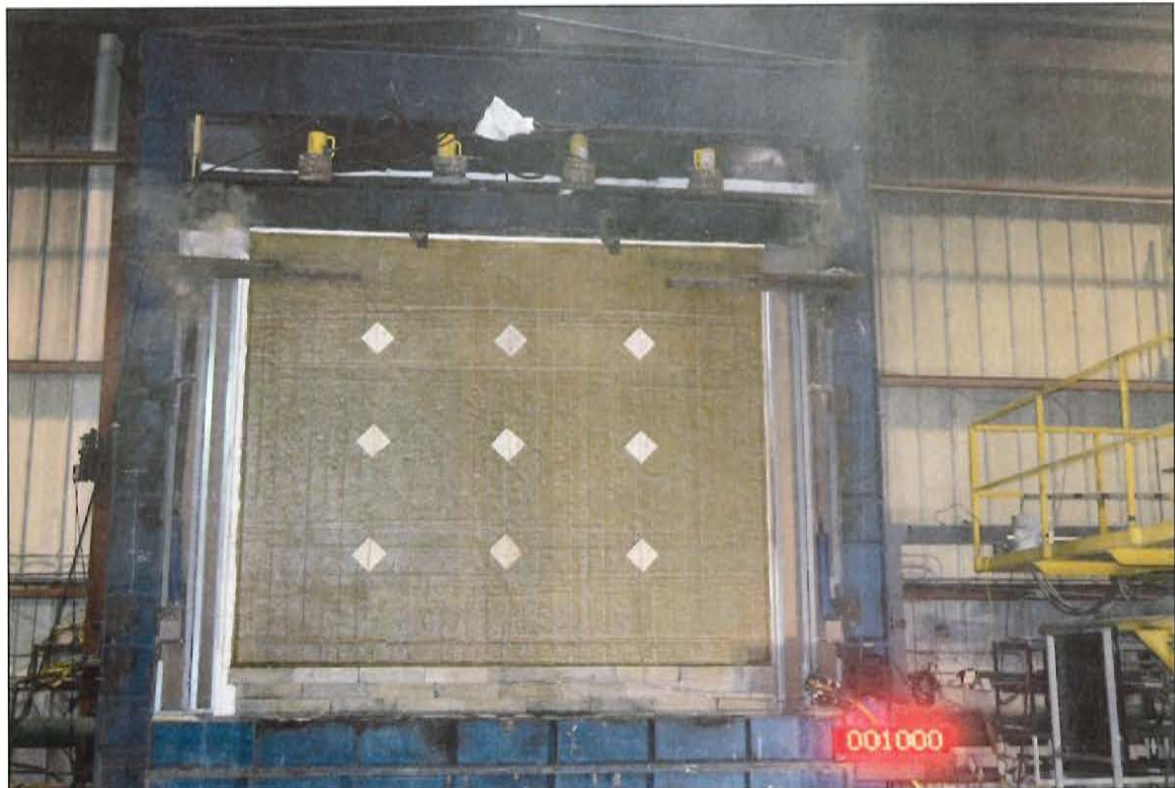
Figure C-4. Unexposed Side of Serial No. 4001b Wall Assembly 10 min into Test.
