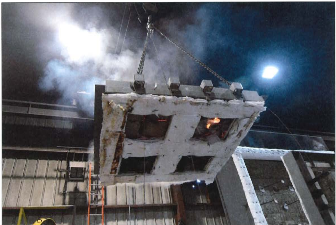
Figure B-6. View of Exposed Side of Samples during Removal from Furnace
