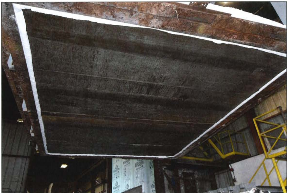
Figure C-2. Exposed Side of Serial No. 4001a Floor Assembly prior to Testing.
