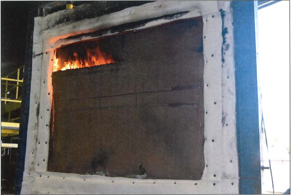
Figure C-9. Exposed Side of Serial No. 4001b Wall Assembly prior to Hose Stream Test.
