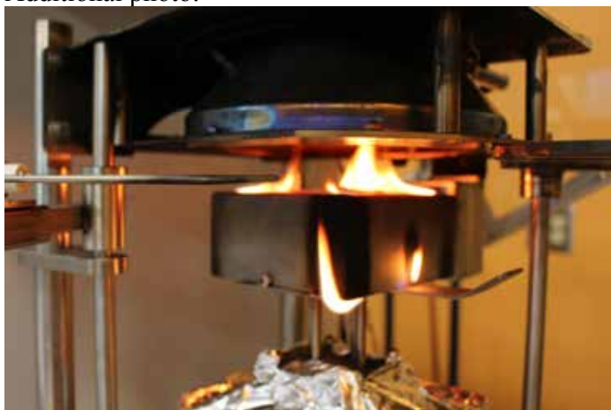
Figure 6. Photo of samples of 1001a dripping and burning under the frame.
