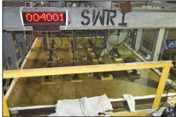
Floor panel at 40 minutes into test. Hydraulic cylinders providing continuous 40 lb/ft 2 load
