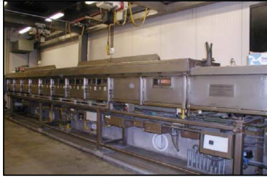
Steiner Tunnel used to run E84 test
