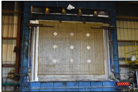
Wall panel sample used in E119 test
