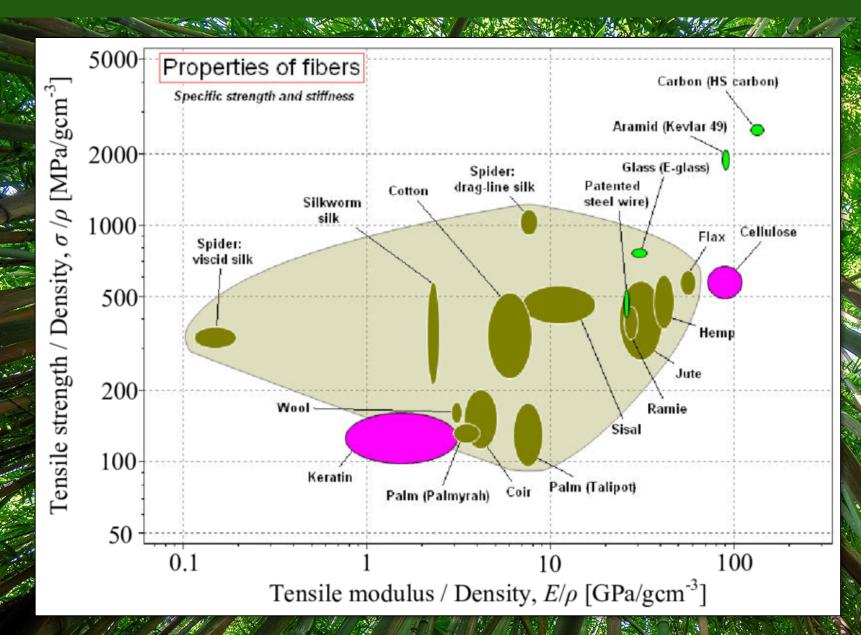
Ashby plot comparing the position of natural fibers against synthetic fibers with respect to specific tensile properties.
