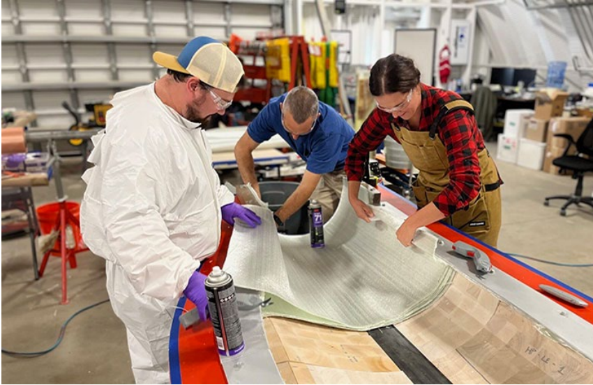
After optimizing it in the lab, the NREL team used their new PECAN resin to glue together a 9-meter wind turbine blade made with fiberglass composites and a balsawood core in NREL's Composites Manufacturing Education and Technology Facility. Photo by Troy Boro, NREL
