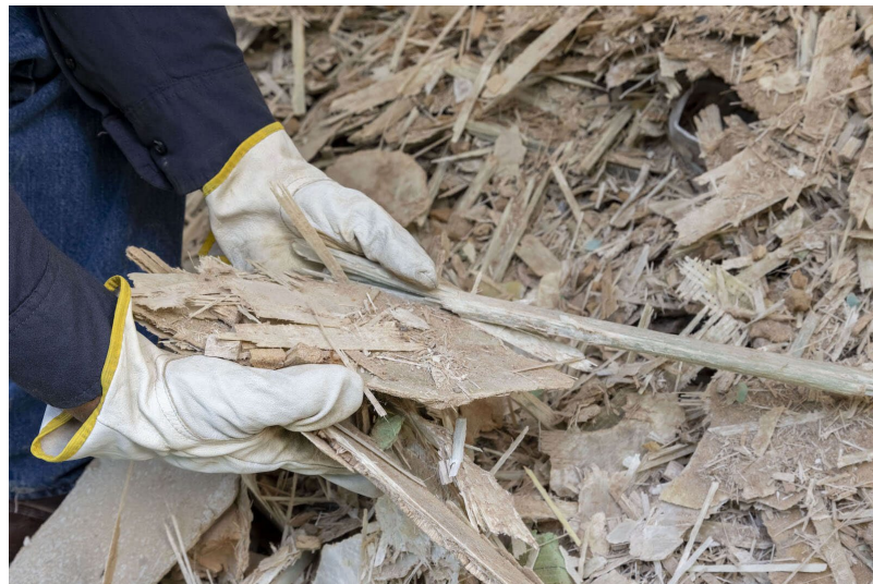
Final product that is realized when the mechanical recycling process is complete in Veolia's blade recycling process. Photo from Veolia
