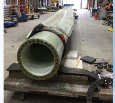
Blade Prep for Testing
