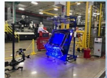
Digital Image Correlation (DIC) for fiber orientation
