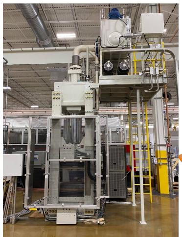
Fast acting press being enhanced with shuttle system to enable shorter cycle times.
