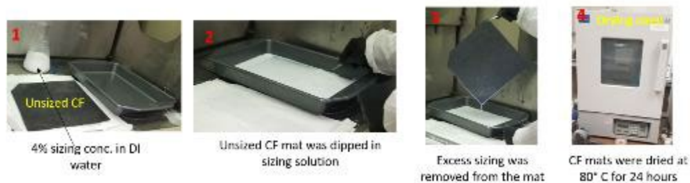
Figure 22. Sizing process description
