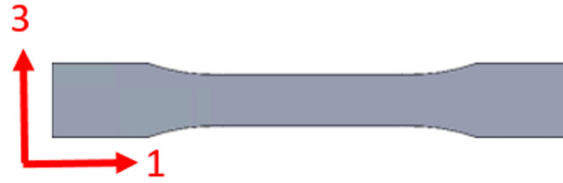
Figure 40. Tensile coupon for mechanical characterization in the 1-direction.
