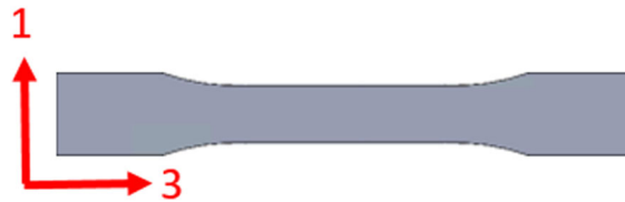
Figure 48. Tensile coupon orientation for characterization in the 3-direction.
