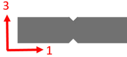
Figure 84. Shear coupon orientation for the 1-3 plane characterization.
