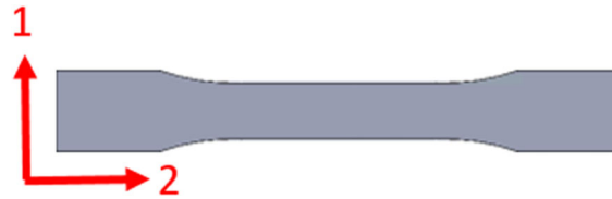
Figure 76. Tensile coupon orientation for the 2-direction characterization.
