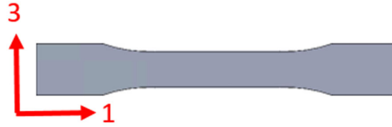
Figure 72. Tensile coupon orientation for the 1-direction characterization.
