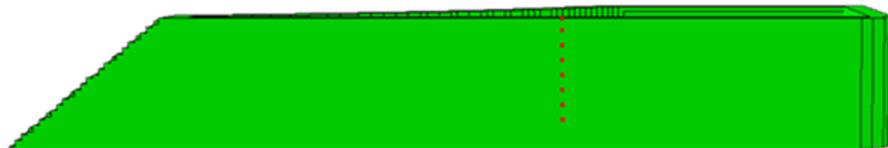
Figure 131. Layer locations in the curved wedge used to extract time-temperature history.
