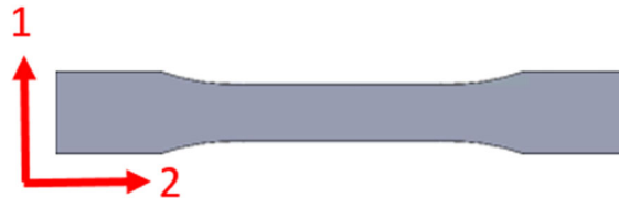
Figure 44 Tensile coupon orientation for the 2-direction characterization
