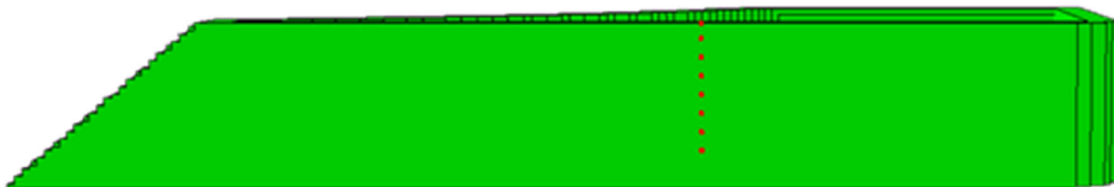
Figure 144. Layer locations in the curved wedge used for extracting time-temperature history.
