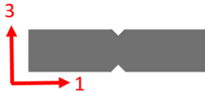
Figure 52. Shear coupon orientation for the 1-3 plane characterization.
