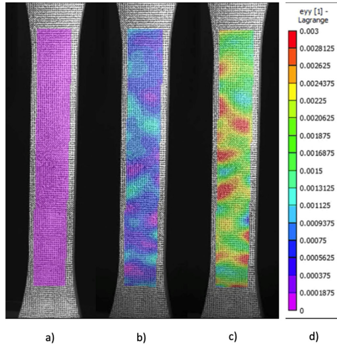
Figure 45. Strain field developed in the load direction at different instants of time. a) before the load application b) when strains start to develop c) just before failure d) strain field distribution.
