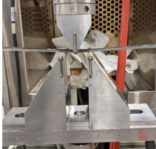
Figure 32: Flexure sample test setup using 3-point bending test fixture with a 33.9mm span.
