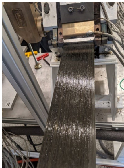
Figure 26: Kevlar ® /VZL-36D prepreg exiting the impregnation die.
