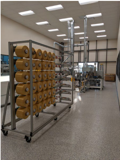
Figure 24: Overview image of the prepreg tape line's 48 position creel (left) and fixed bar fiber spreading unit (right).
