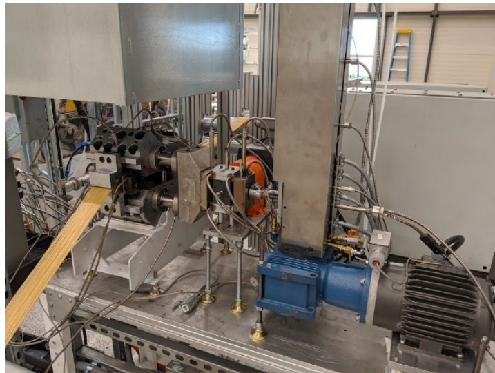
Figure 25: Overview image of the prepreg tape line's extruder, melt pump, and impregnation die.
