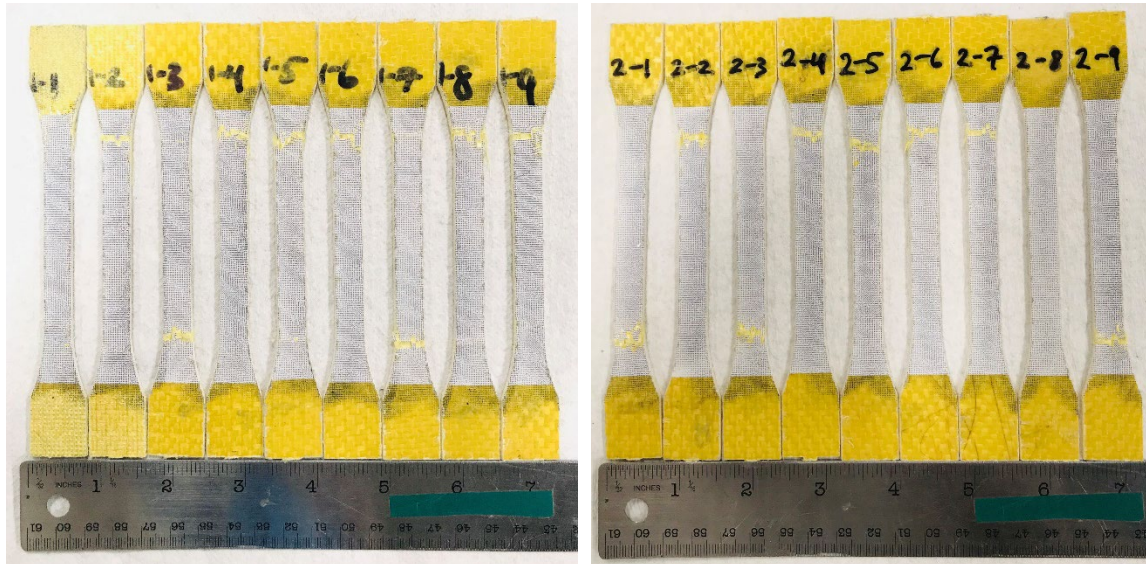
Figure 6: Failed tensile samples from laminates T-P-1 and T-P-2
