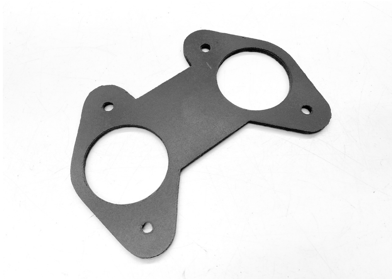
Figure 11 Test part made with CMC binder carbon fabric and Evonik D390 PA613 powder
