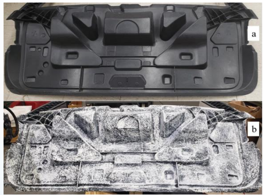
Fiber orientation prediction and measurement using Digital Image Correlation (DIC)
