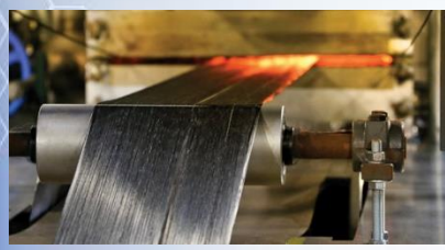
Textile PAN Carbon fiber → Spar Cap Pultrusion
