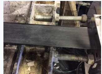
Textile PAN Carbon fiber → Spar Cap Pultrusion
