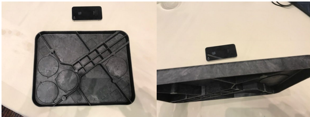
Figure 1. Tool design and parts; Representative multiple-process tool used to produce long fiber injection-compression and extrusion-compression part. The part features thick, thin ribs, thin/thick base areas, channel variations, and characteristics that provide understanding of material flow through the cavities.
