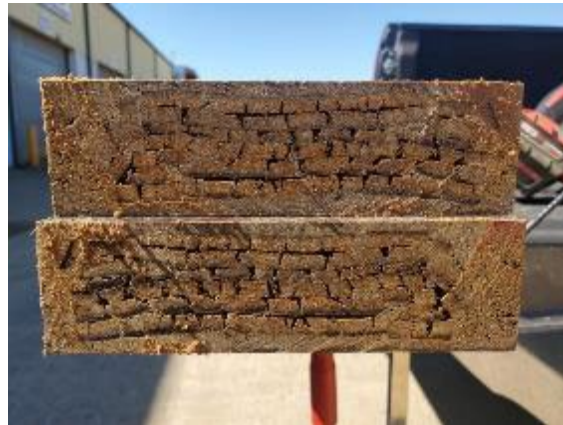
Figure 29. Edge view of the Resource Fiber panels used in the testing. The bamboo strips core and the jacket made from ECM bamboo-PP are clearly seen. The core is not fully wet out with the resin as can also be seen
