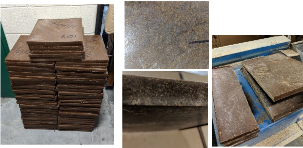
Figure 25. Some of 200 panels of bamboo-PP made via ECM at the UT FCMF. The panels were edge trimmed to size to fit in the deck mold (tool) in line.
