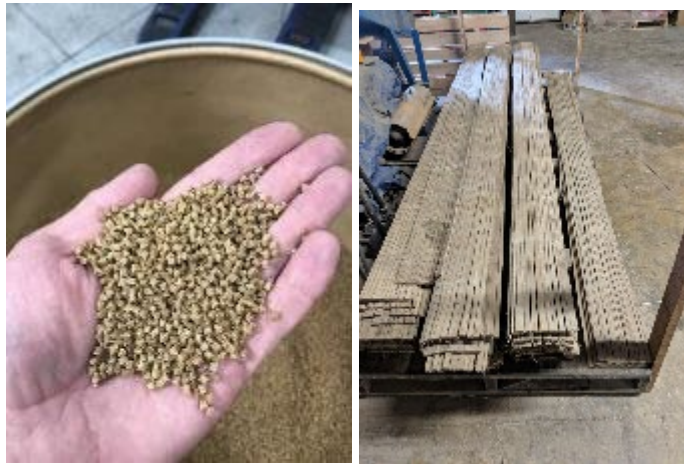
Figure 24. Simple blending 50% conditioned bamboo fiber with PP and long solid strips of bamboo core 1.125" thick:
