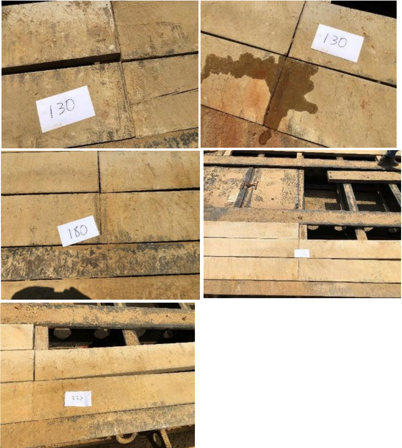
Figure 32. Illustration of survivability of bamboo decking for cycles 130, 180 and 225 respectively, Same comments about no indications of failure progression were observed.
