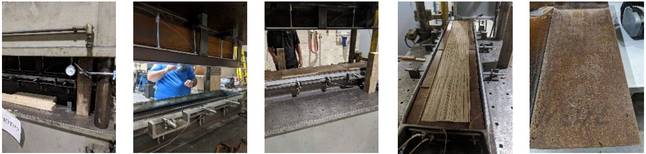
Figure 26. Various steps of processing 4 feet bamboo-PP panels at UT on the Dake press
