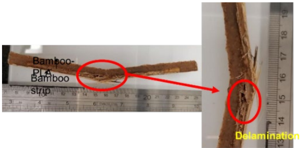
Figure 8. Representative failure modes in flexural loading of bamboo-PLA/bamboo strip
