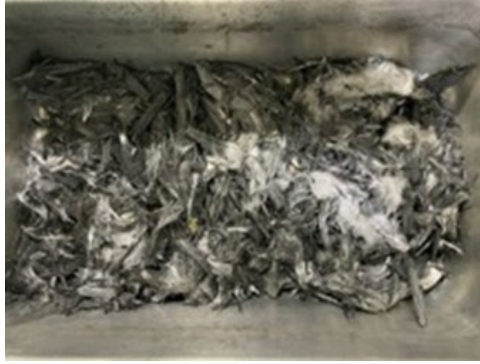
Figure 9. Fiber recovered after sonication indicating noticeable char removal although more impurities remaining when compared versus high temperature burn off.
