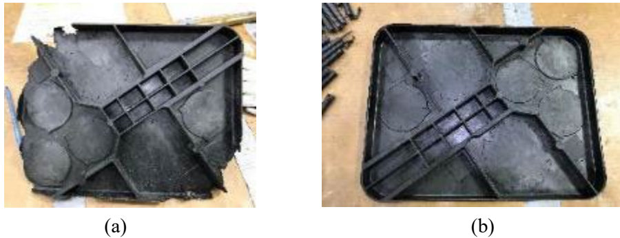
Figure 26. Representative battery tray cover parts made from rCF-PA66 and rCF-epoxy. The parts look very similar for both materials. (a) short shot in IM of rCF-PA66 and (b) fully filled part.
