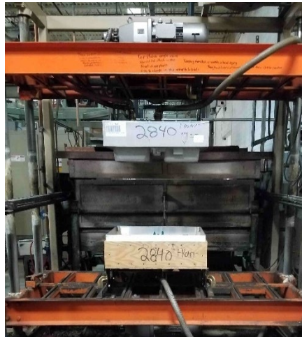
Figure 24. Vacuum thermoforming machine and tool used to mold the John Deere door panel.
