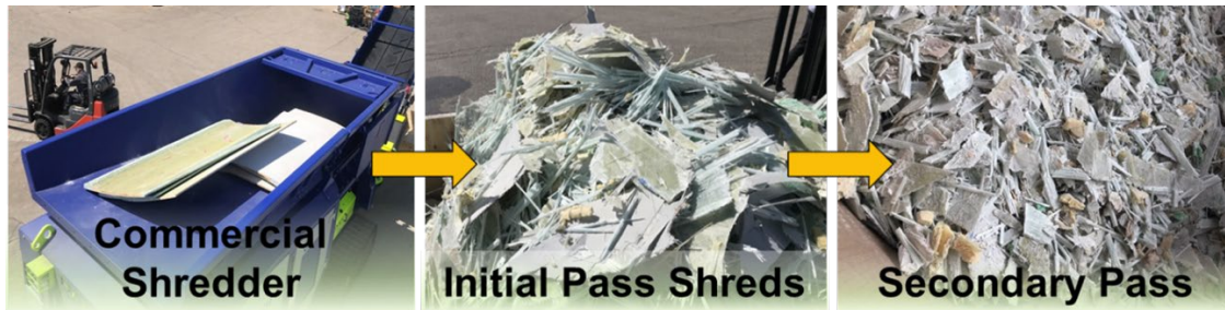
Figure 1. Shredding sequence for converting wind blade end of life materials, originating from GE Renewable Energy, into Thermolyzer™ feedstock.
