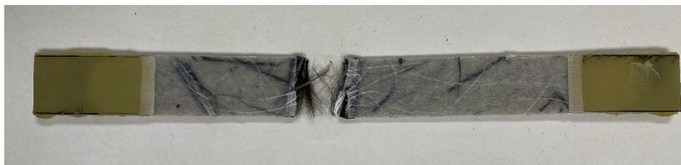
Figure 13. Observed specimen fracture in tensile testing reveals failure through fiber separation in remaining char coated bundles.
