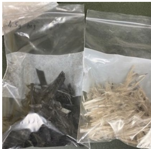
Figure 8. Char covered pyrolyzed fiber before (on left) and after (on right) high temperature burn off in ambient atmosphere.
