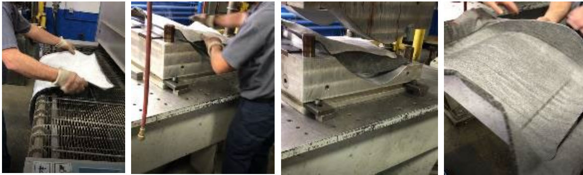
Figure 23. Processing sequence of infrared (IR) heating of the rCF-PA66 mat and transfer to the press for compression molding. Left to right: IR heating of rCF-PA66 in conveying oven; transfer heated rCF-PA66 to press (tool); 5-min cycle time and demold; and back side of the part.
