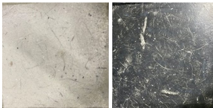
Figure 11. Consolidated LDPE composite test panels after compression molding procedure: burn off fiber panel on left appears white while sonicated fiber panel on right appears black.
