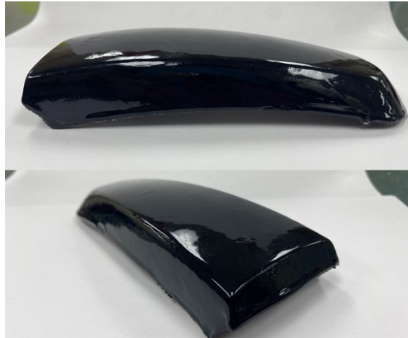
Figure 14. Example bicycle stem geometry molded from LDPE nonwoven mats and burn off rGF after basic polishing and painting.
