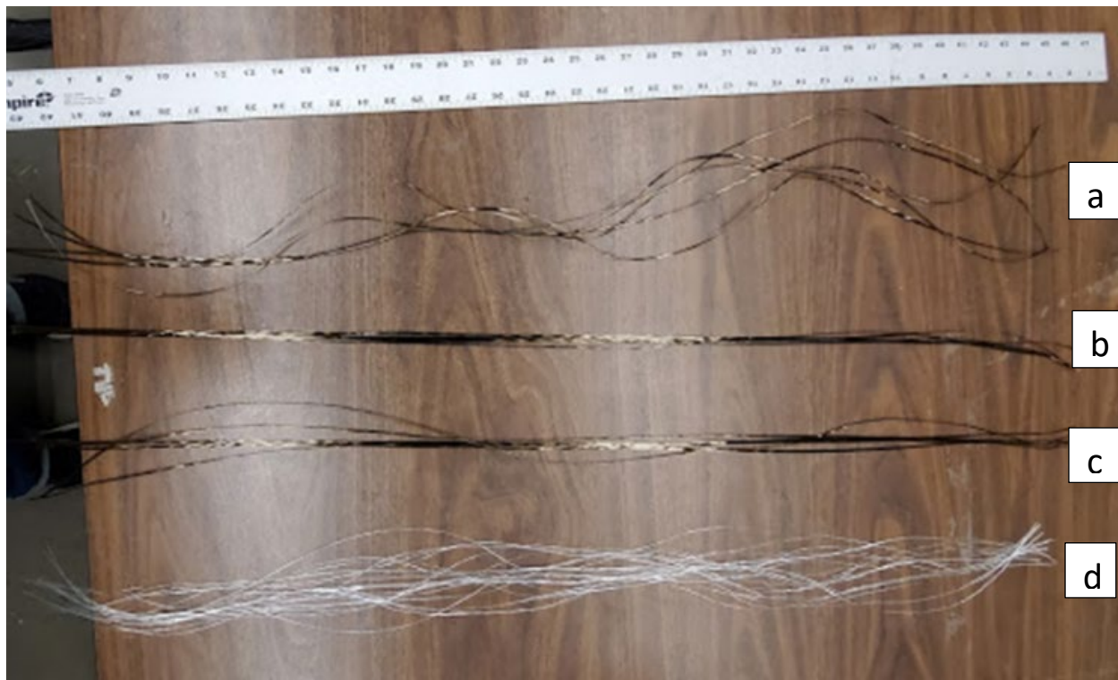
Figure 6. Example basalt fiber sized with (a) Michelman Hydrosized® HP302 (b) Mafic 5X1, (c) Michelman E-Sizing and (d) ME1960 glass fiber tow strands before infusion with epoxy and vinyl ester resin systems.
