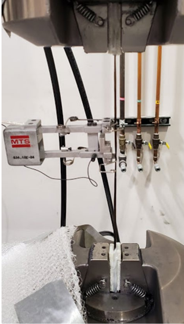
Figure 9: Example mechanical testing setup of tow strand.
