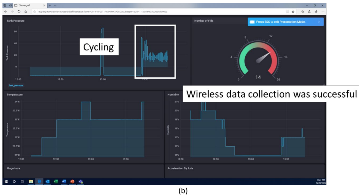
FIGURE 45: READOUTS OF DATA RECORDED BY THE WIRELESS MEASUREMENT DEVICE. PRESSURIZATION DURING THE AUTOFRETTAGE AND BURST OF ONE VESSEL IS SHOWN ON (A), AND THE PRESSURE OSCILLATIONS FROM THE PRESSURE CYCLING OF THE OTHER VESSEL IS SHOWN IN (B)
