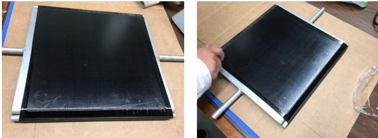
FIGURE 6: FLAT PANELS OF UNIDIRECTIONAL COMPOSITE FABRICATED BY ORNL USING FILAMENT WINDING ON A FLAT PADDLE
