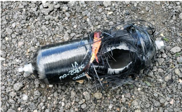
FIGURE 12: CYLINDRICAL BURST MODE IN A STEB VESSEL SUBJECTED TO A HYDROSTATIC BURST TEST
