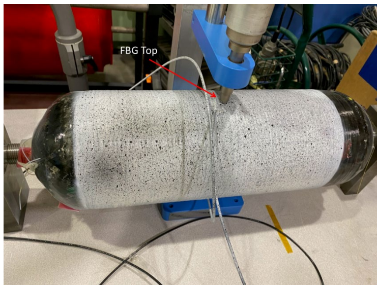
FIGURE 29: PICTURE OF THE IMPACT SITE AND THE FBG BOUND TO THE TOP OF THE VESSEL, ADJACENT TO THE IMPACT SITE. NOTE THAT THE FBG IS ORIENTED TO MEASURE HOOP-DIRECTION STRAIN
