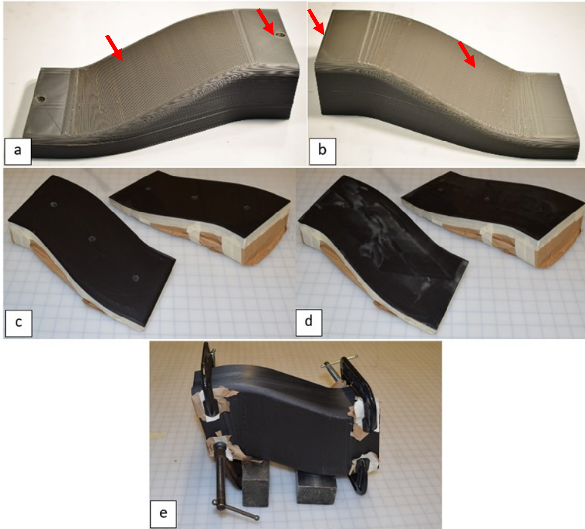
Figure 32 Duct 1 was printed as two halves and experienced ironing on the surfaces indicated by the red arrows (a, b), had holes drilled in the bottom bonding surface (c), was bonded together (d) and clamped to cure (e).
