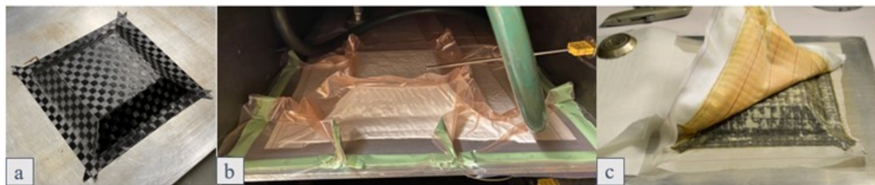
Figure 12 Composite manufacturing process including: (a) the layup of prepreg on Pyramid A; (b) loading the vacuum bagged composite into the autoclave; and (c) removal of the consumable materials used during processing.
