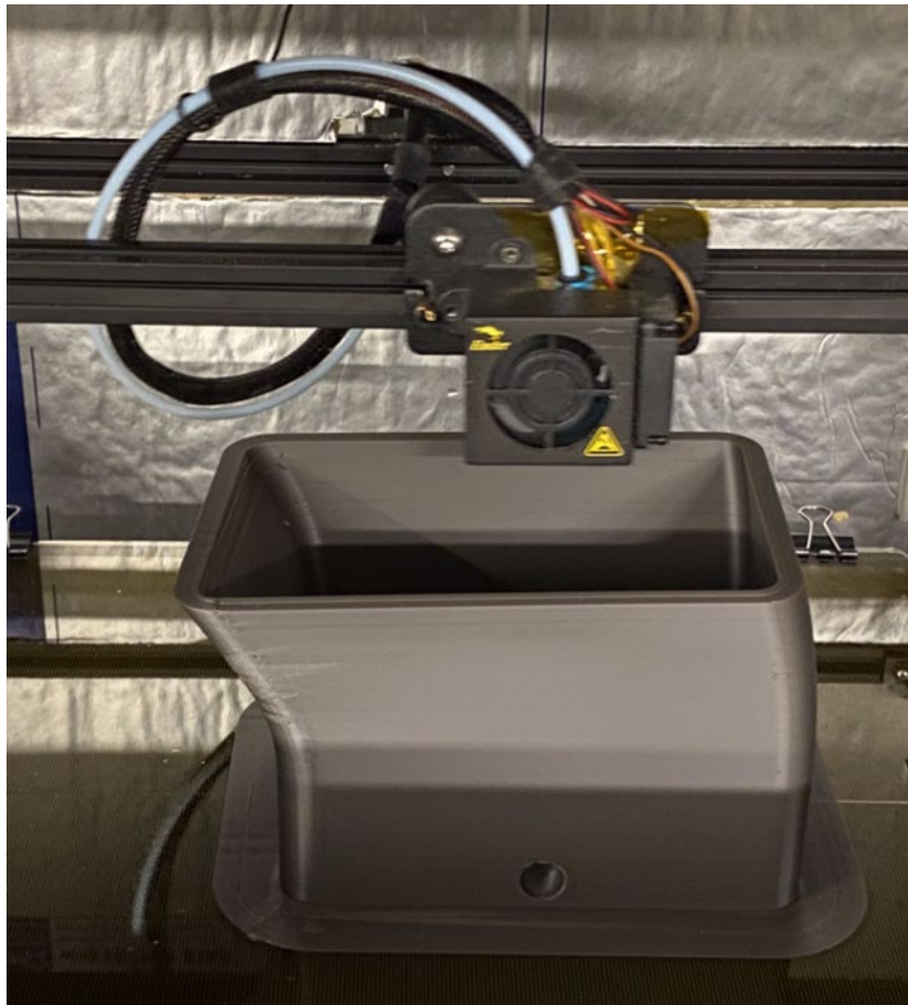
Figure 27 Hollow bent duct printing process for Tool 2.
