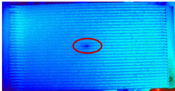
Figure 60 - IR image of 3D printed sample 3 with the nozzle located 25 mm below the defect and the shop air flow on (defect circled in red)
