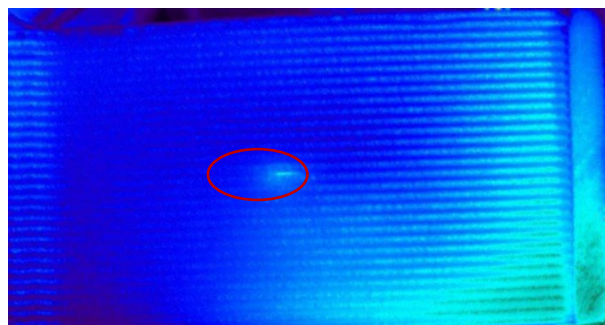
Figure 56 - IR image of 3D printed sample 3 with the nozzle located 25 mm to left of the defect and the shop air flow on (defect is not visible)
