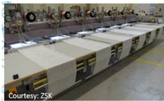
Figure 77. Commercial Scale ZSK TFP Fabrication Setup
