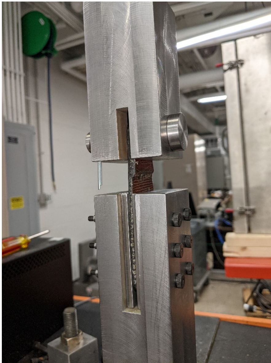
Figure 53. Clip Bracket in Instron Load Frame
