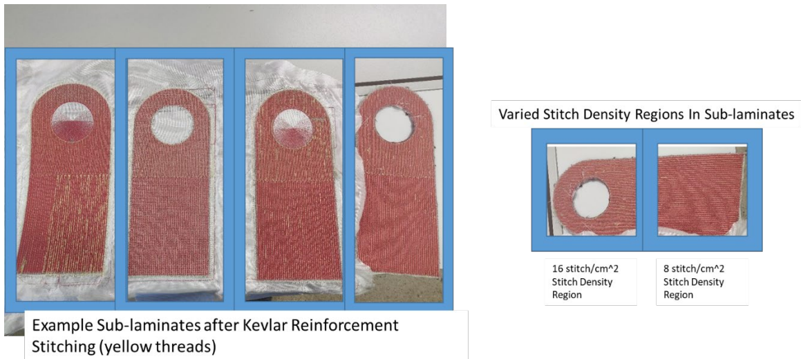
Figure 33. Example Lug Sub-laminate Preforms, and Stitch Density Diagram
