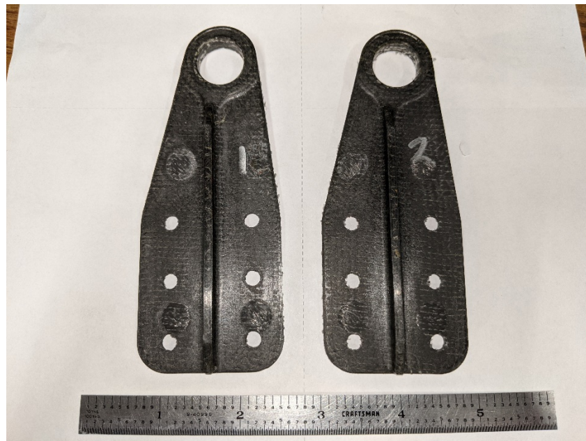
Figure 52. Clip Bracket after De-Molding and Machining
