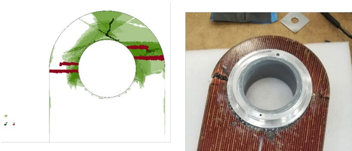
Figure 73. Computational Model Predicted Failure of a Hard Point Model against Experimental Failure
