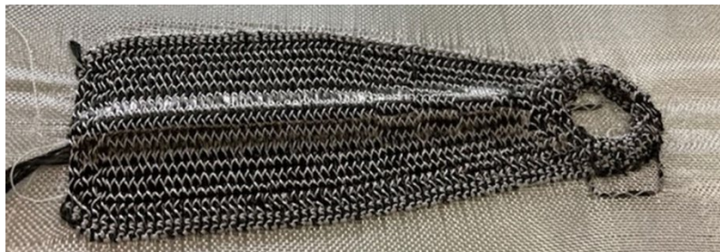
Figure 51. Clip Bracket Spine TFP Preform
