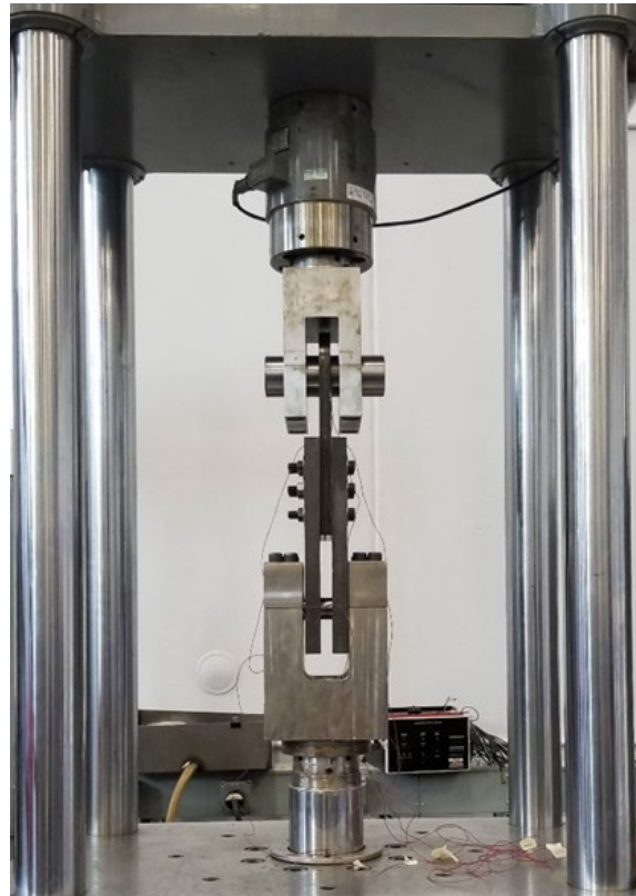
Figure 39. Image of Test Specimen in MTS Hydraulic Load Frame Prior to Testing
