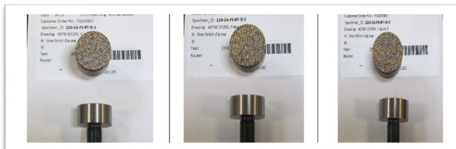
Figure 8. Sample ILT Adhesive Failures at Interfaces
