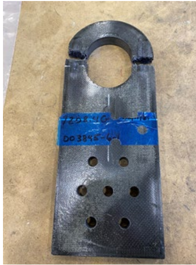
Figure 40. Failed IM7 Plain Weave Lug Geometry
