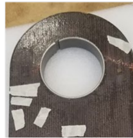
Figure 41. IM7 TFP Lug Sample Failure Images
