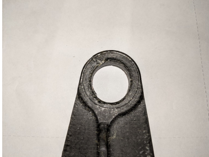
Figure 54. Failed Clip Bracket Surface
