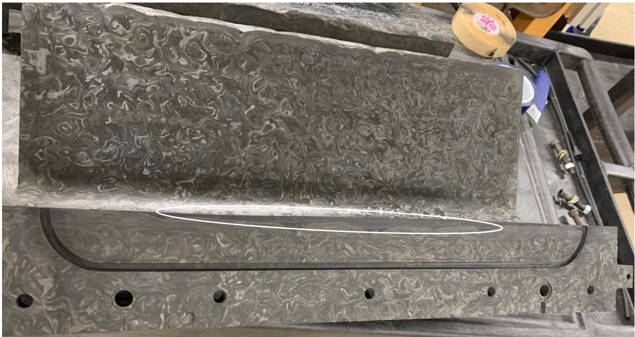
Figure 15. Machined subscale tool, assembled (top) and single half (bottom). Circle indicates area where tool filler was applied
