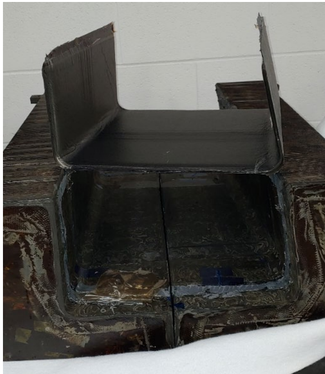
Figure 24. Cured c-spar part made from master-approach tooling
