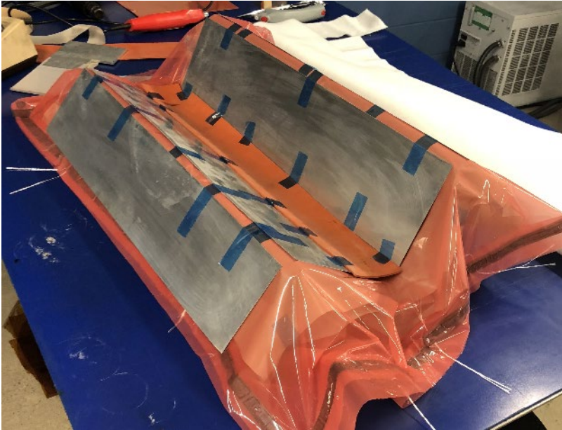
Figure 12. Release film and caul plates installed prior to cure
