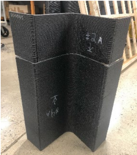
Figure 10. Right half of BAAM print after bonding, approximately 24 inches tall
