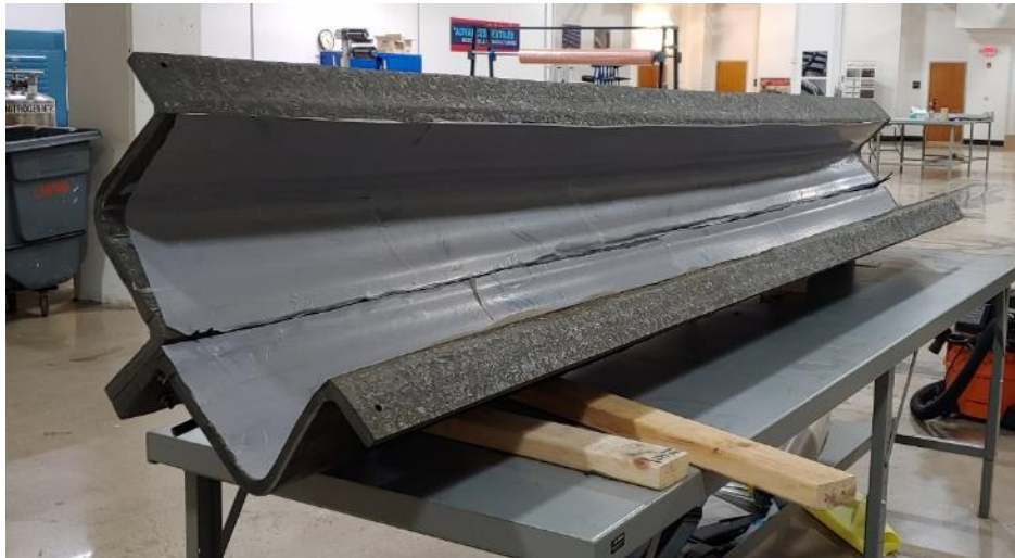
Figure 28. Machined tool with release film applied
