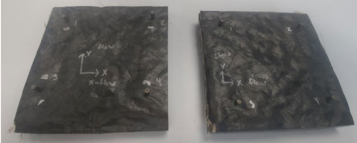
Figure 7. Laminated tooling panels for CTE check
