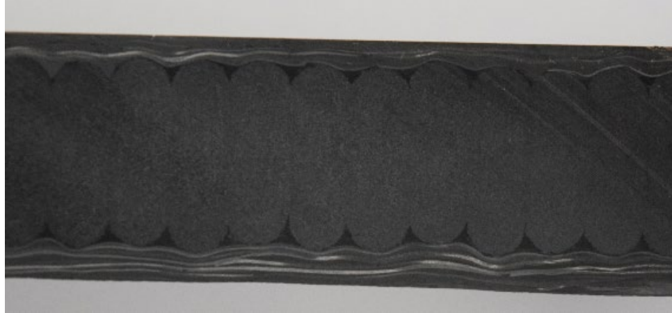
Figure 5. As-printed coupon cross-section after heating
