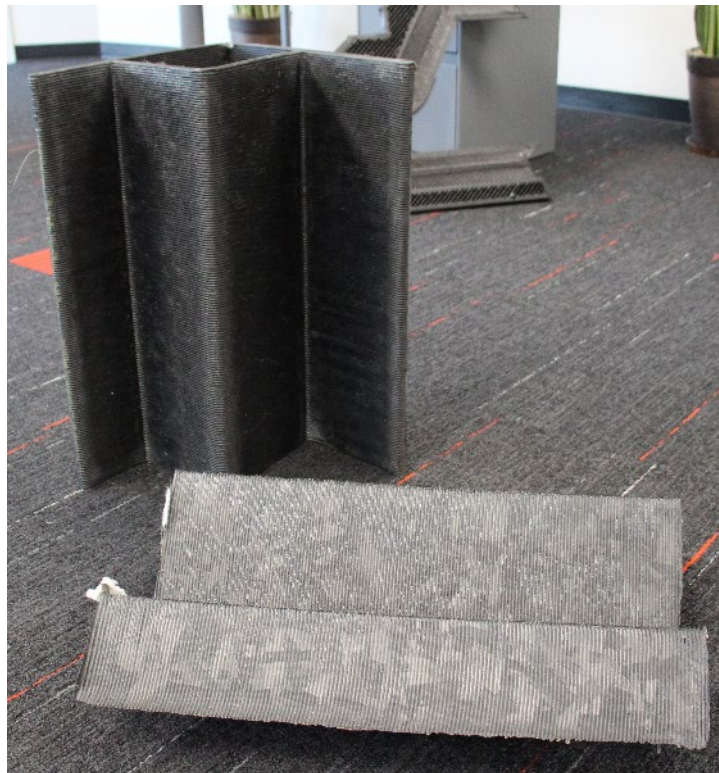
Figure 22. Cured tool half demolded from BAAM master
