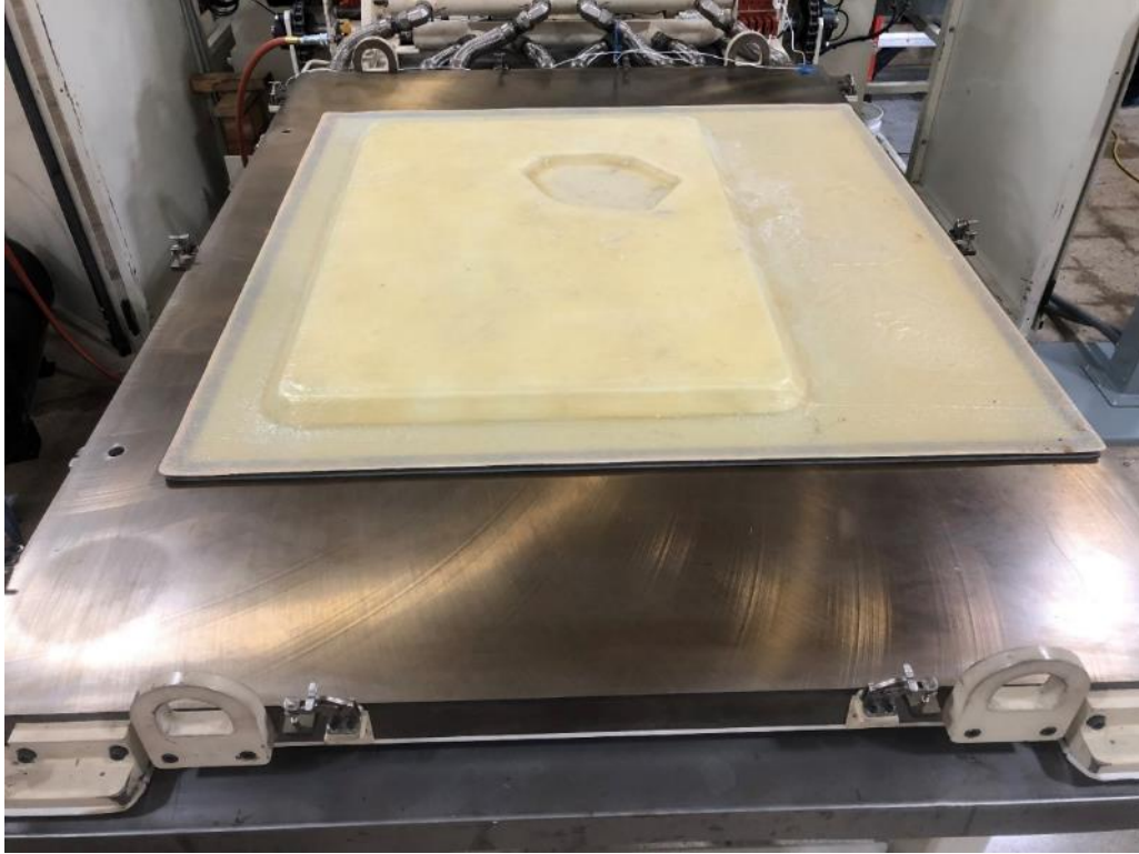
Figure 16. Composite Caul Covering Preform and Machined Tool Sitting on RapidClave® Tool Plate
