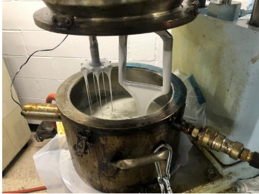
Figure 6. Snap Cure Resin after Mixing Resin, Hardener, Catalyst, and Defoaming Agent
