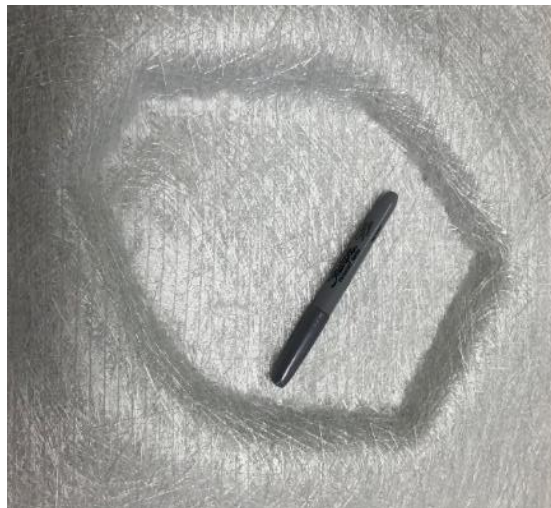
Figure 9. MultiMat Fabric formed against a preforming mold (marker used for size reference)
