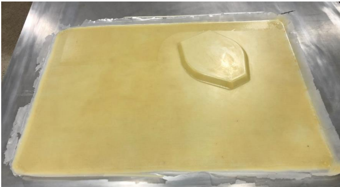
Figure 17. Composite Door Panel Molded using RapidClave® before Trimming
