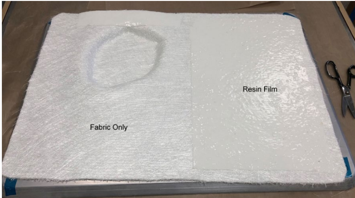
Figure 11. Fabric Reinforcement with Resin Film
