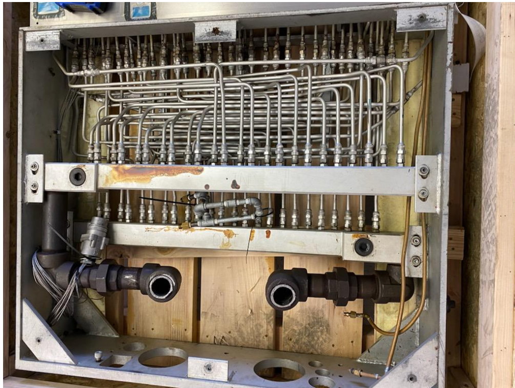
Figure 1. Typical plumbing for an integrally-heated tool
