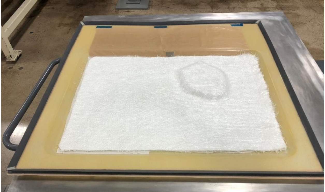
Figure 15. MultiMat Preform Applied to Resin Film on Composite Caul
