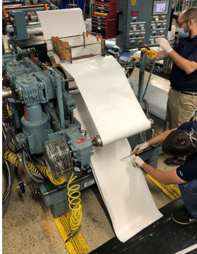
Figure 7. Sheets of Resin Film being produced on Film Line
