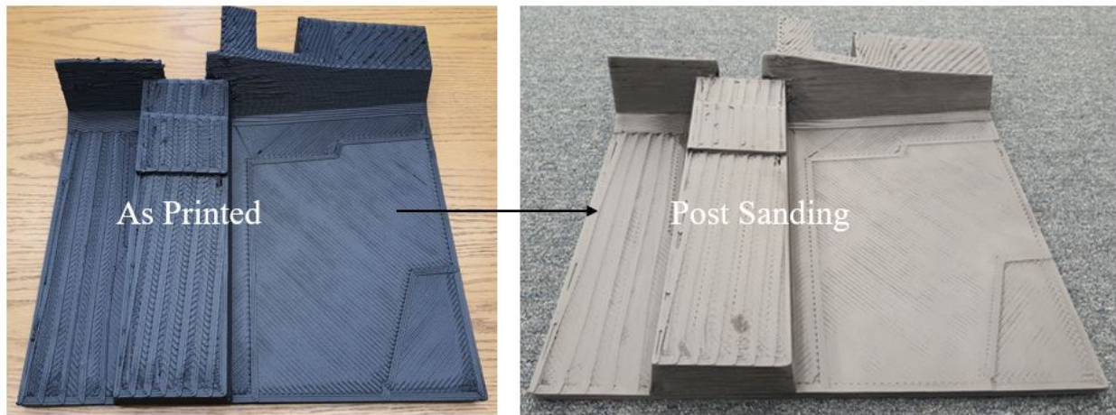
Figure 12 Printed Floor Tool Before and After Sanding (Apparent color change is due to lighting conditions)
