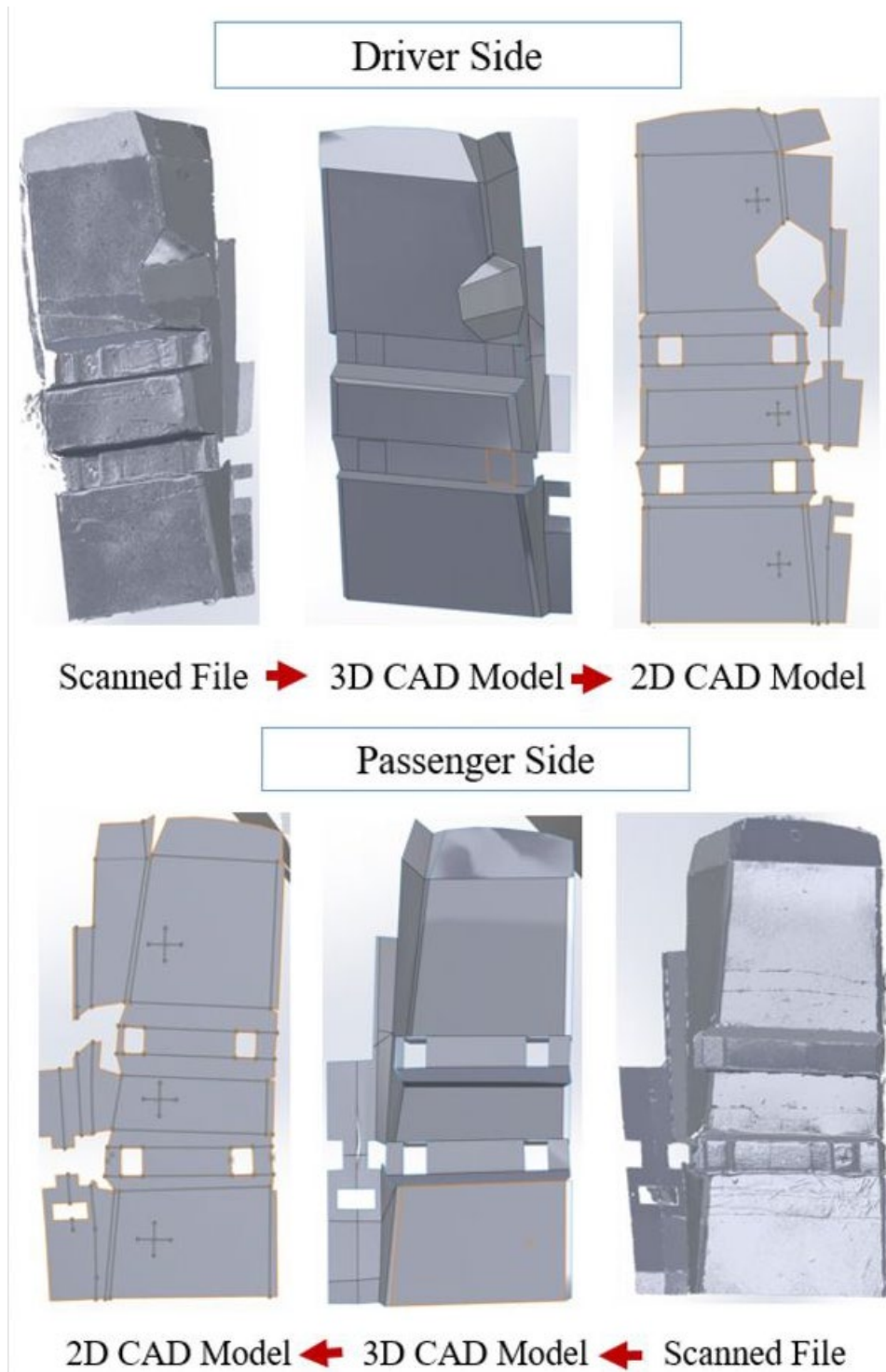
Figure 6 Floor Scans Rebuilt and Flattened
