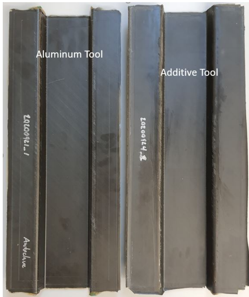
Figure 7 Baseline Hat Stiffeners Processed in Autoclave
