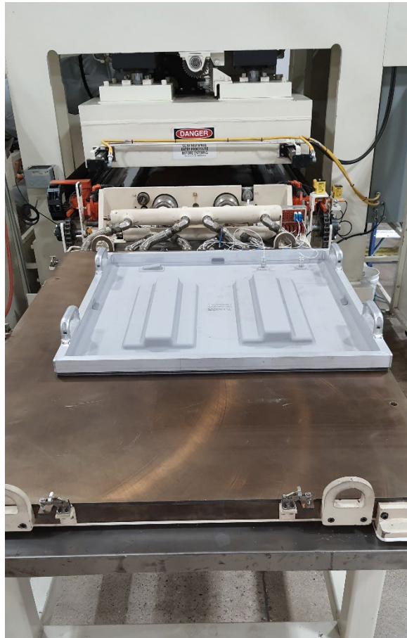
Figure 8 Torr Bag Vacuumed Down to Hat Stiffener Tools on RapidClave® Platen
