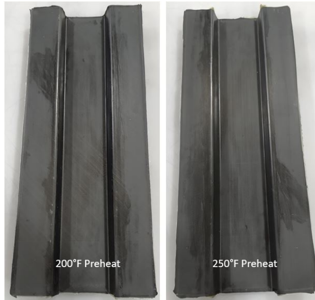
Figure 12 Additional Hat Stiffeners: 200°F and 250°F Preheats
