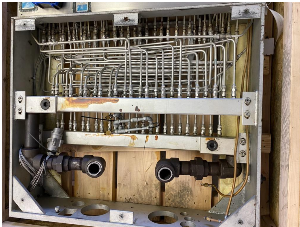
Figure 1 Typical Plumbing for an Integrally-Heated Tool
