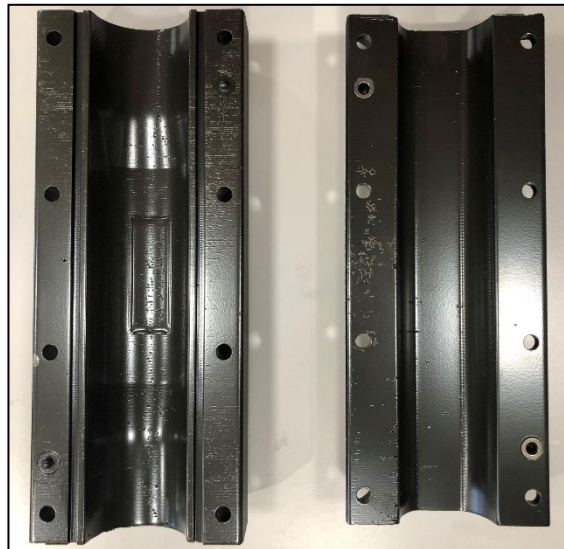
Figure 17. Demo Tube Form Mold Coated with TruDesign Epoxy Sealer
