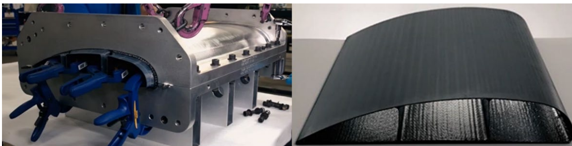
Figure 26. Trailing Edge Bond Toolset for Aeroshell Overwrap and Internal Structure Integration
