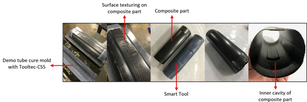
Figure 24. Demo Tube Cure Mold Final Assembly
