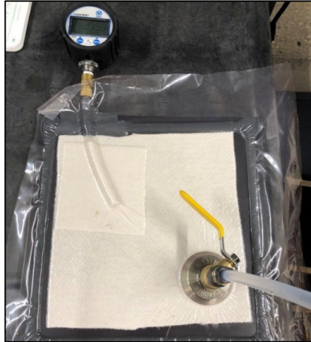
Figure 12. Surface Vacuum Bag Configuration on Square Trial Panel
