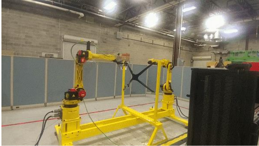
SSA-ACUT scan on robotic platform
