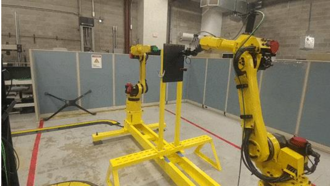
SSA-ACUT scan on robotic platform
