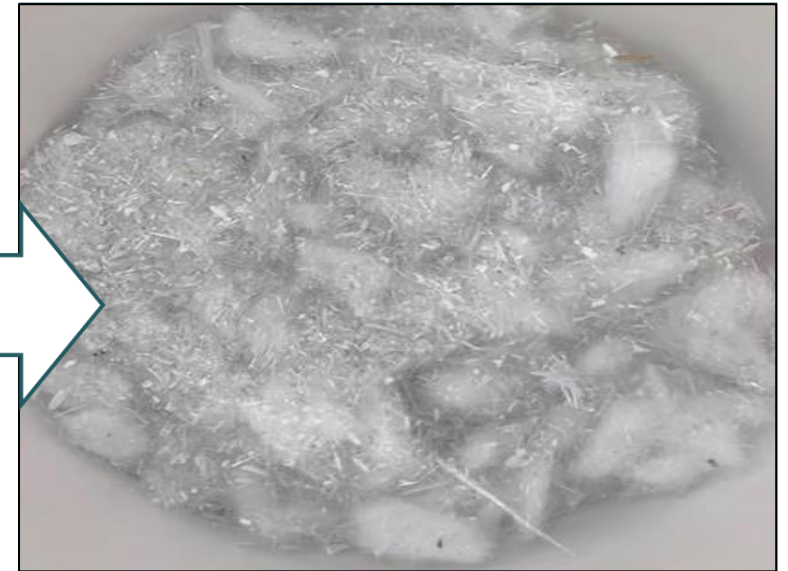
Carbon Rivers Thermochemically Recycled Fiberglass
