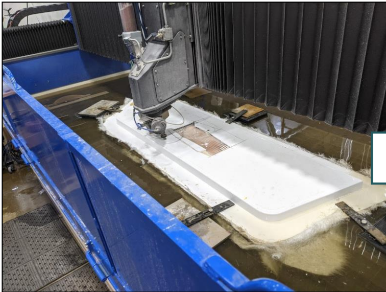
ORNL Waterjet Cutter Cutting Failed Boat Hull Sandwich
