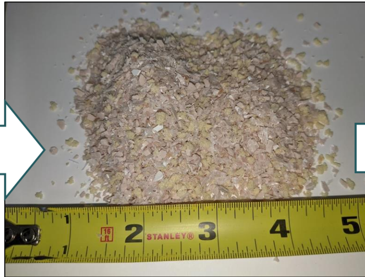
ORNL Shredded Sandwich into Granulate Pieces Less than 0.25" Diameter
