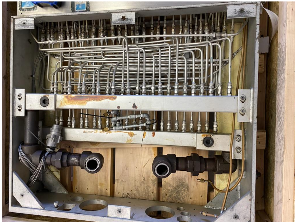
Figure 1. Typical plumbing for an integrally-heated tool
