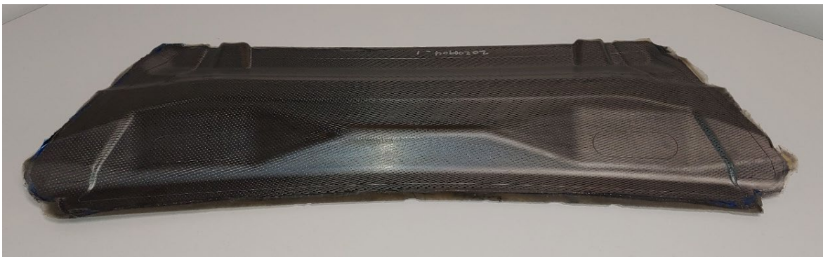
Figure 11. Cured CYCOM EP2750 Volkswagen part
