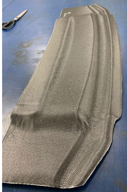
Figure 8. Preshaped ply stack fabricated in a single debulk operation
