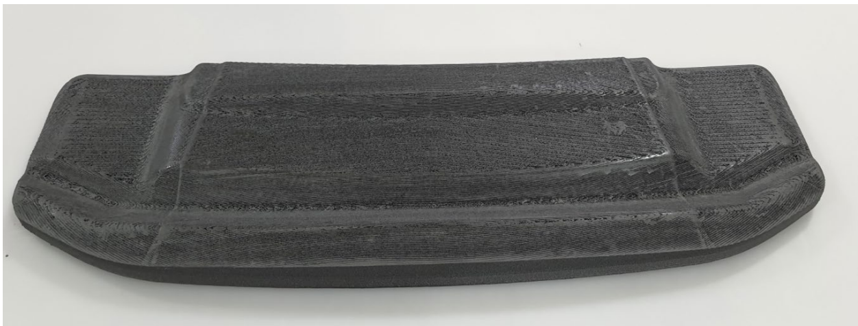
Figure 9. Additively manufactured draping tool
