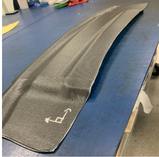
Figure 7. Preshaped ply stack fabricated ply-by-ply
