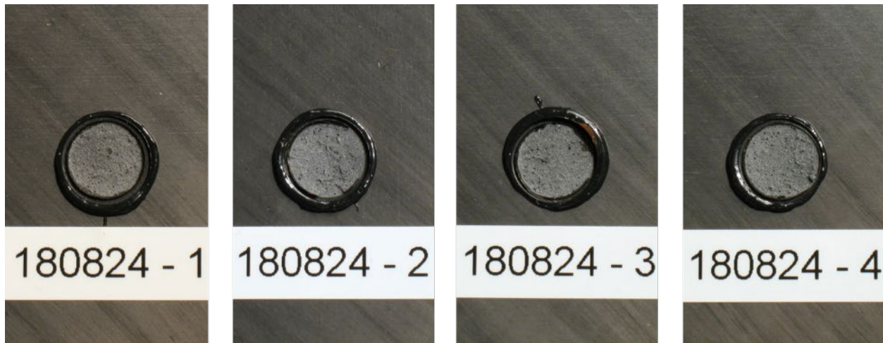
Figure 106. Failure surfaces of non-IMR composite/Betamate PATTI specimens.
