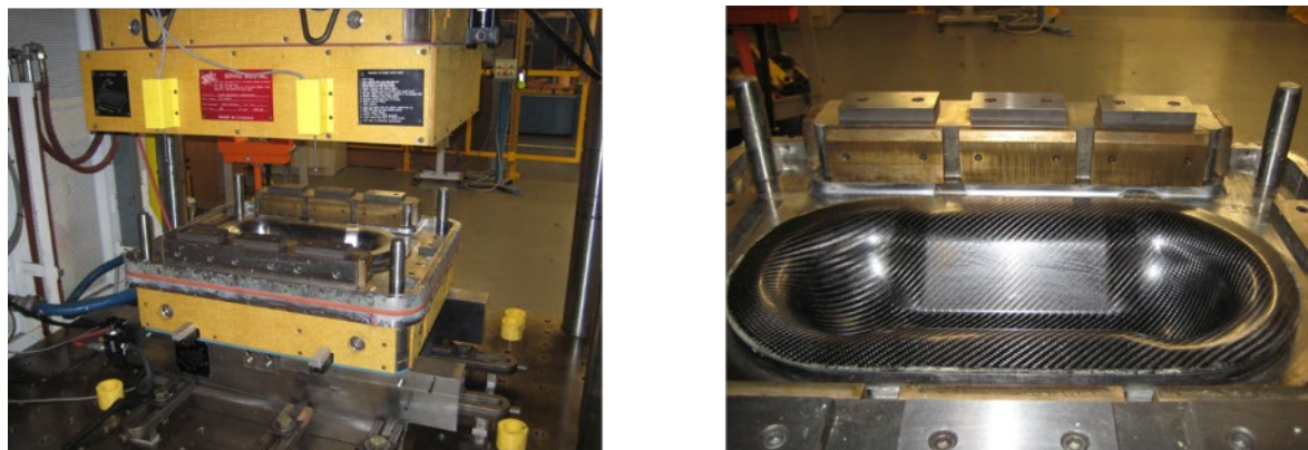
Figure 2. Double dome compression molding tool.
