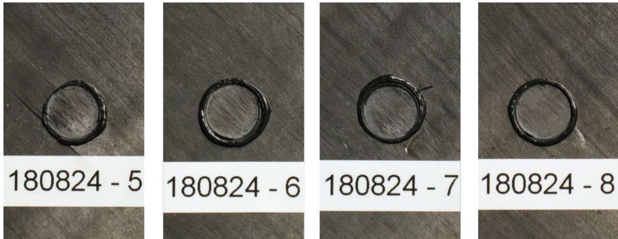
Figure 107. Failure surfaces of composite with IMR/Betamate PATTI specimens.
