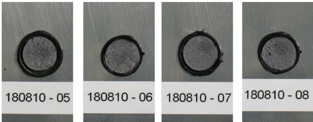
Figure 96. Failure surfaces of IPA-cleaned aluminum/Betamate PATTI specimens.
