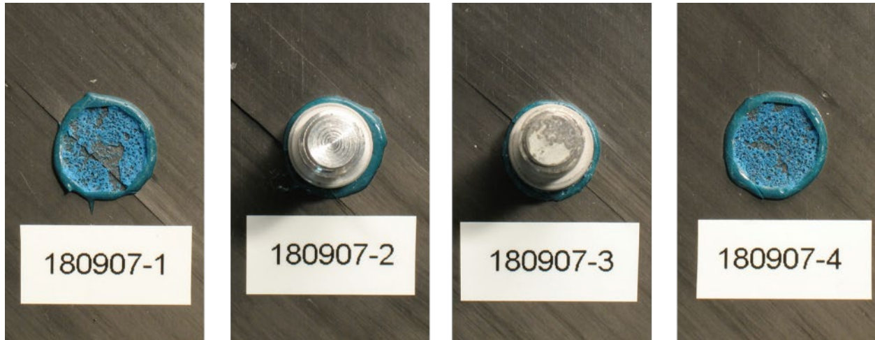
Figure 108. Failure surfaces of non-IMR composite/1K-Flex PATTI specimens.
