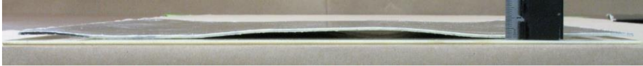
Figure 76. Edge view of panel LMG-061617-02, warpage approximately 8 mm.
