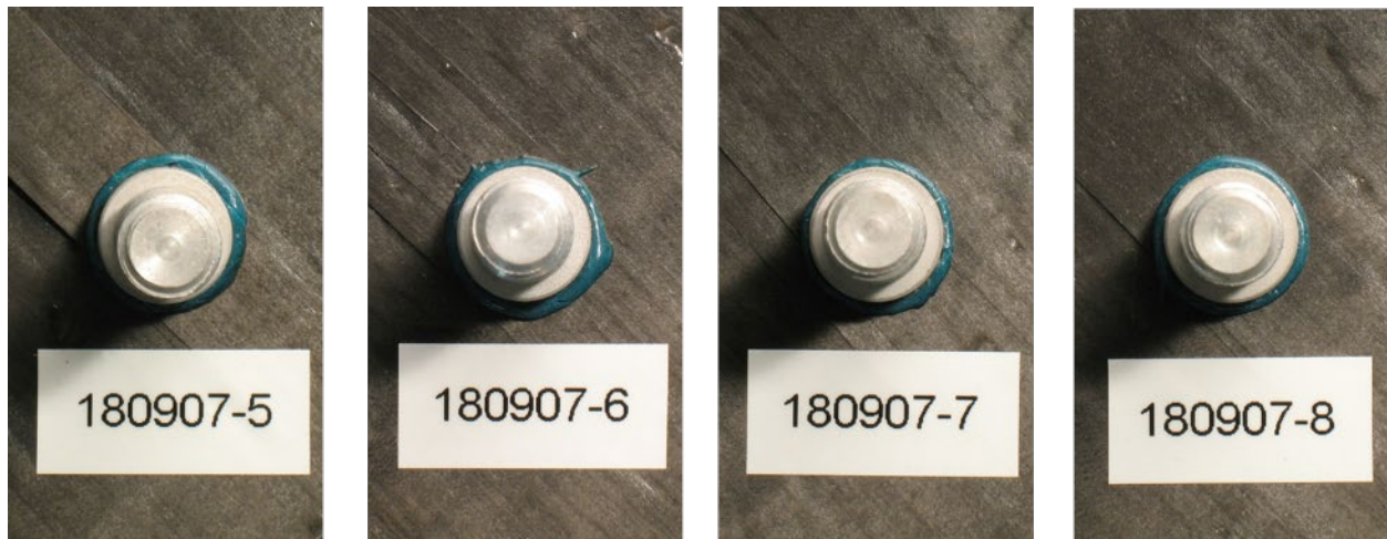
Figure 109. Failure surfaces of composite with IMR/1K-Flex PATTI specimens.
