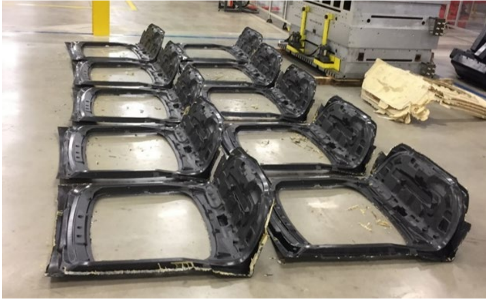
Figure 139. Liftgate inner panels molded at IACMI Corktown (SURF).
