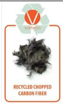
Vartega then recovered the fiber from the scrap material that was not created into a liftgate. Michelman and TechmerPM compounded the material with 10% carbon fiber, so it could be utilized in injection molding capacities.
