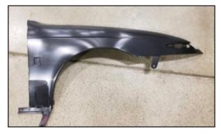
The new material with recycled carbon fiber was injection molded into fenders. The resulting fender has 60% lower embodied neergy than if using the original carbon fiber, which is the current traiditional method. These results open new doors for cost savings for creating a lighterweight material for automotive production.
