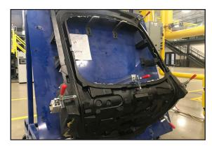
A technical project with Dow and Ford created a novel composite material, which has achieved part level material performance such that Ford is willing to declare it acceptable for specification on future vehicle platforms. The material was compression molded into liftgates to validate.
