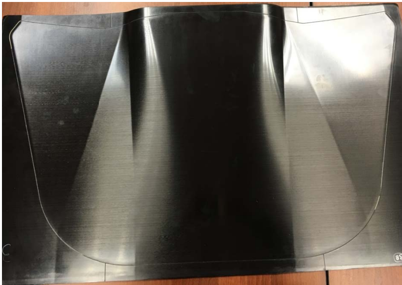
Figure 22. Examples of minimal rework LIT molded panel (untrimmed)
