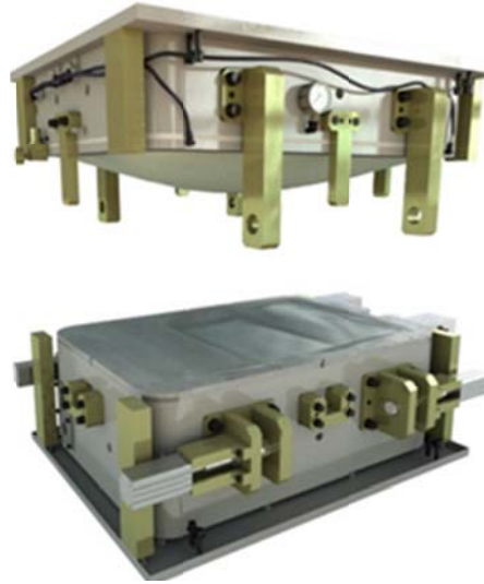
Figure 6. RocTool Light induction tool
