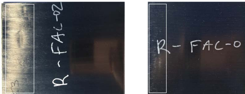
Figure 19. Fiber distortion and dry spots on surfaces of press molded panels
