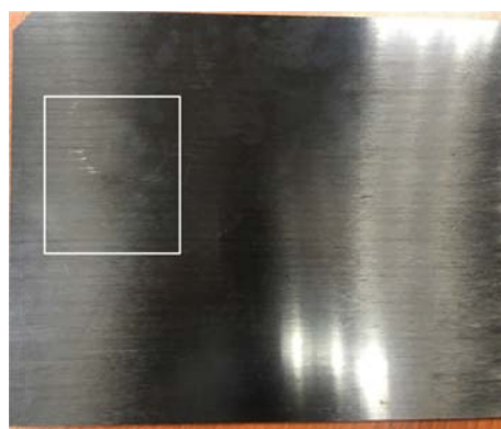
Figure 20. Hairline dry spots on surface of press molded panel
