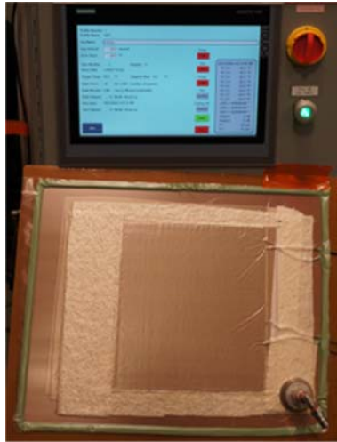
Figure 5. Janicki heated composite light tool
