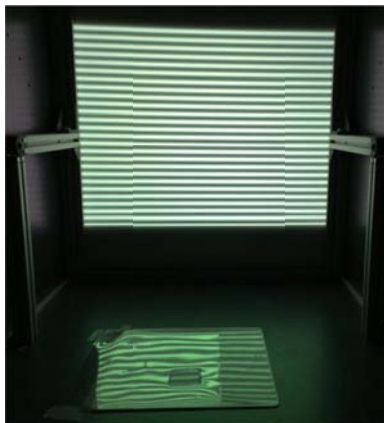
Figure 23. Deflectometry set-up. The grid pattern is projected from the top screen onto a panel below. The reflected pattern on the panel is captured and analyzed by a computer for deformations in the reflections to conclude topography of the surface.
