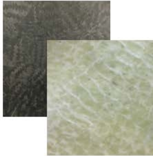
chopped pieces of Renegade prepregs molded after 23 months
