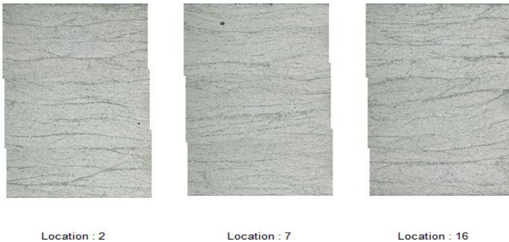
Figure 6. Cross Sections of 901/PX35 ribbon at 3 Locations (Width of View = 1.6 mm)
