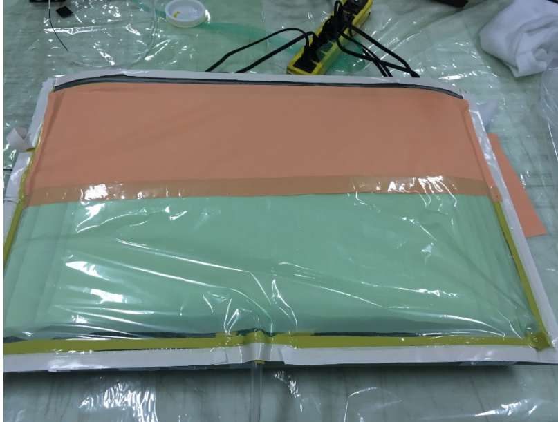
Figure 36: Part with first layer of bagging applied (breather and a second vacuum bag will be applied around this).
