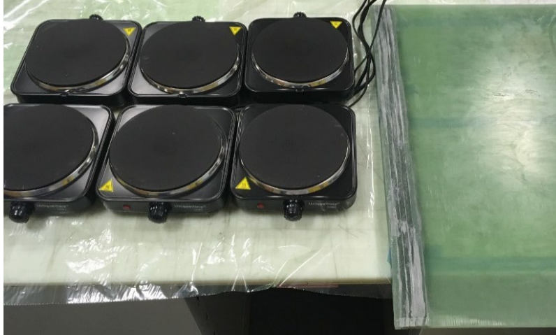
Figure 32: Hot plates used as heating elements for the mold.
