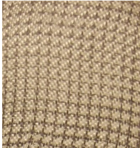
Figure 13: Glass fabric with grid pattern stamped onto it for shearing measurement.
