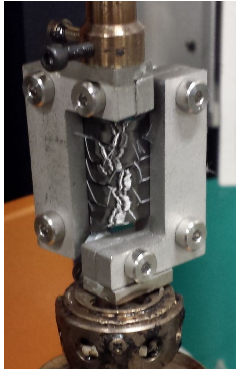
Figure 4: Bending stiffness experimental method for a 0 degree, 0 outside test.
