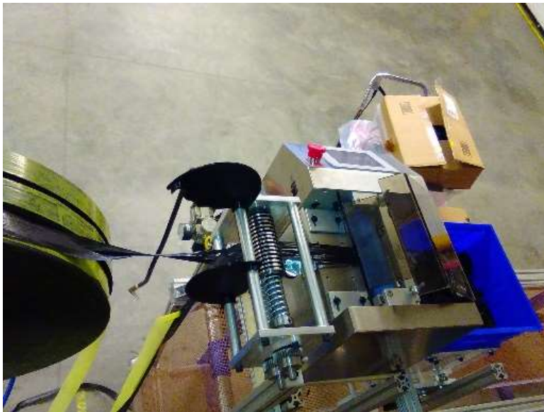
Figure 16 In-line Slitter with Multi-Tow Mounted Directly to Guillotine Chopper
