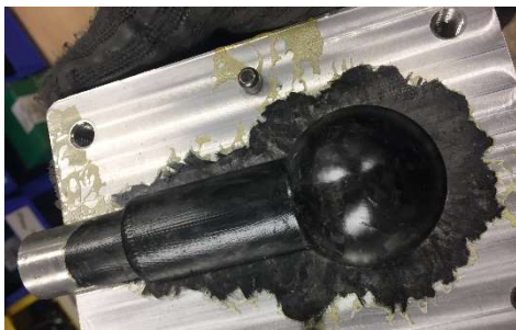
Figure 6 Ball Joint; hollow shaft, solid end
