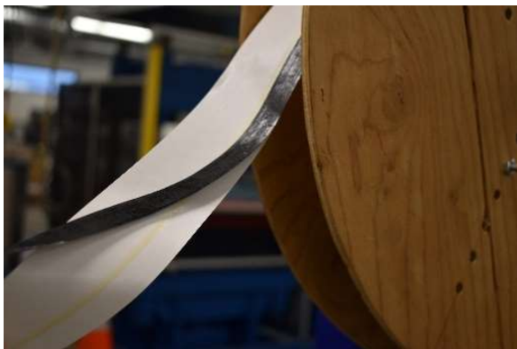
Figure 1 Edge-Trim and Roll Scrap Pre-preg
