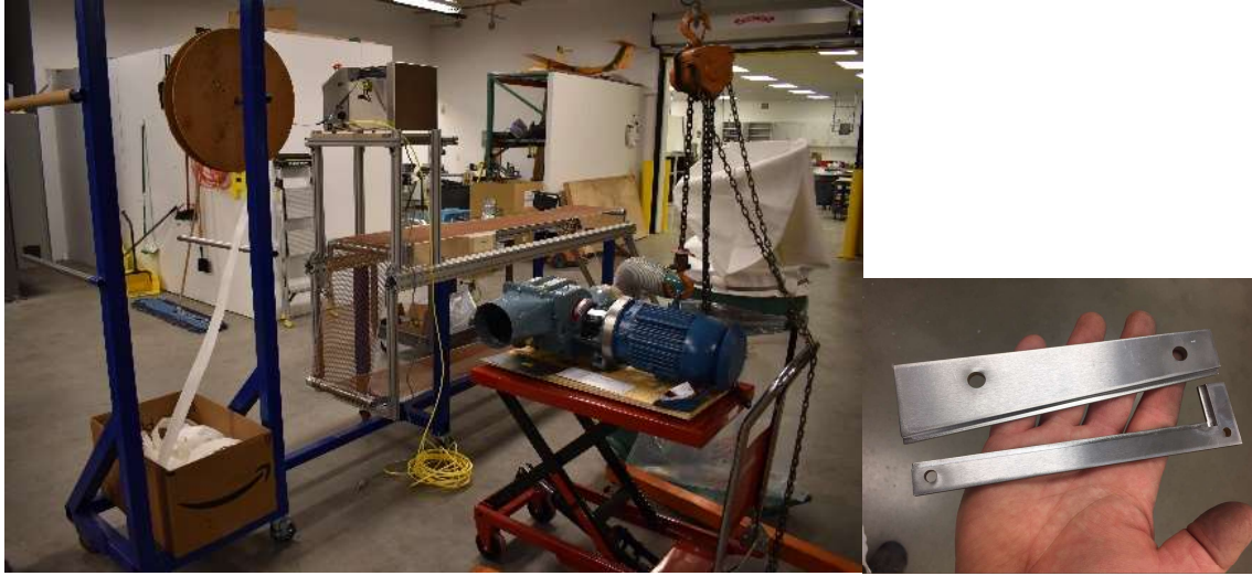
Figure 15 Guillotine Chopper Mounted to Preform Draw Belt
