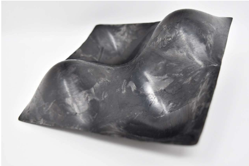
Figure 7 Hyperbolic Paraboloid, High-Flow, High-Deformation
