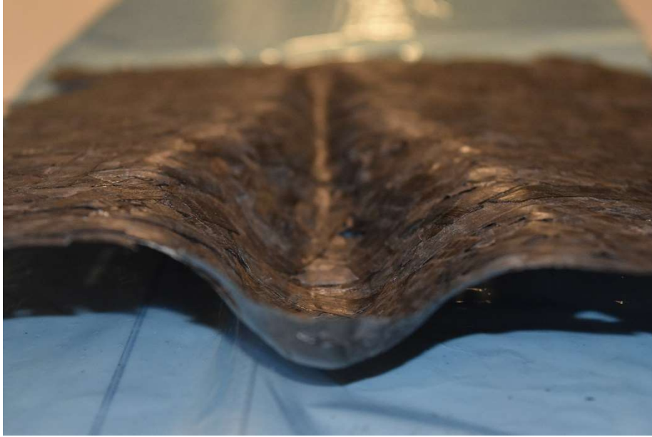
Figure 3 Variable Radius Tapered Preform
