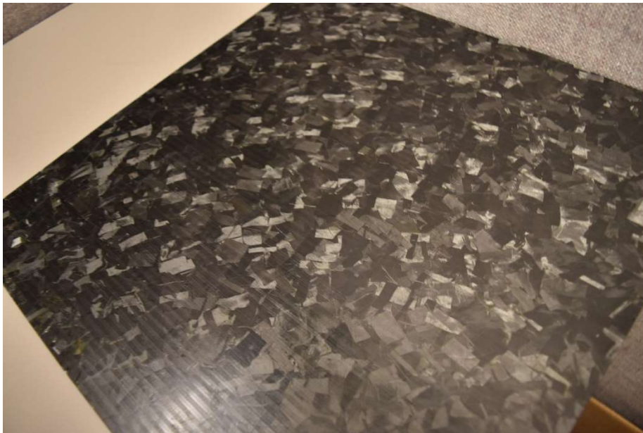
Figure 4 Flat Plate - 0.5 to 12.5 mm Thicknesses Molded
