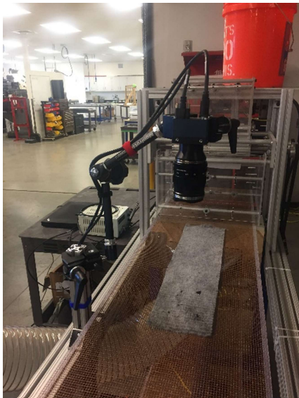
Figure 21 In-Line Non-Contact Chip Coverage Measurement
