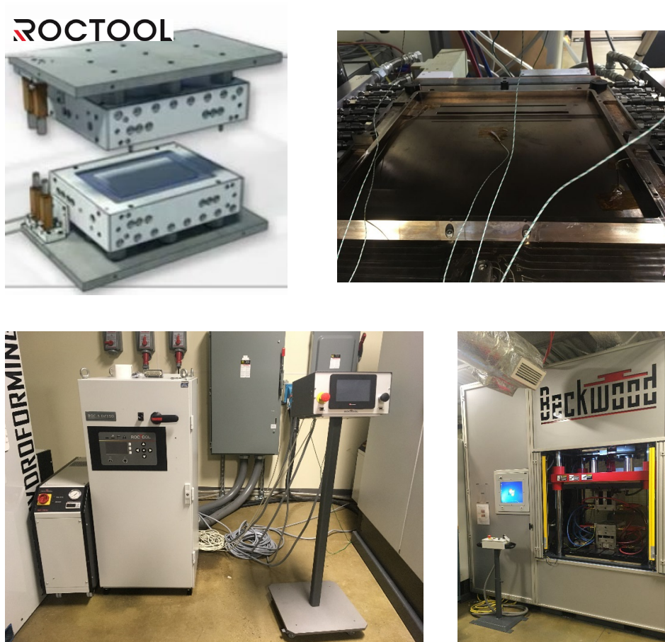
Figure 1. Drawing of the RocTool compression molding tooling (top left), B-side of the tool undergoing temperature mapping with thermocouples (top right), induction generators and control system (bottom left), and the press utilized at Oak Ridge National Laboratory
