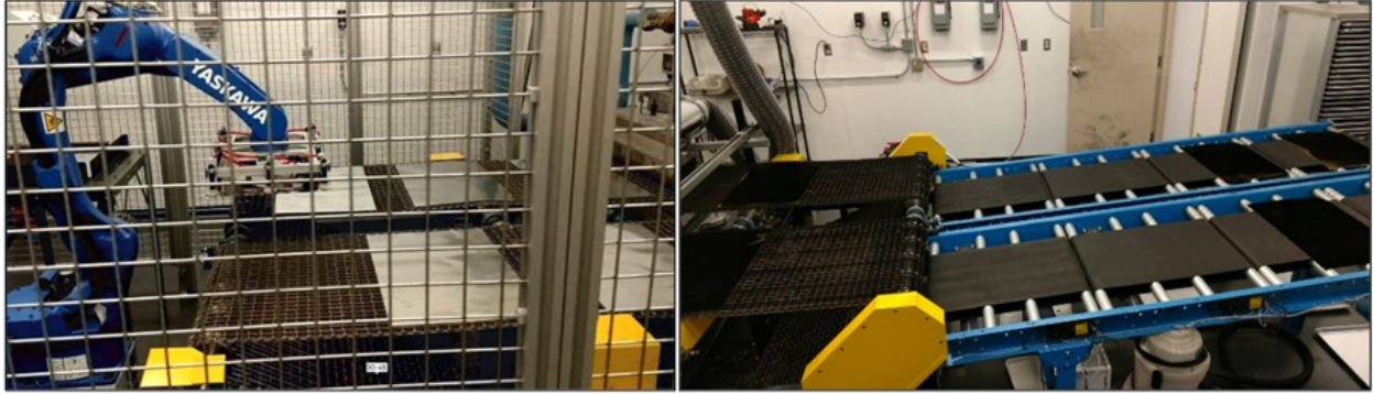
Figure 6. Photographs of the robotic loader and conveyor unloader for VACNT growth substrate and grown VACNT product, respectively. Installed January 2019.
