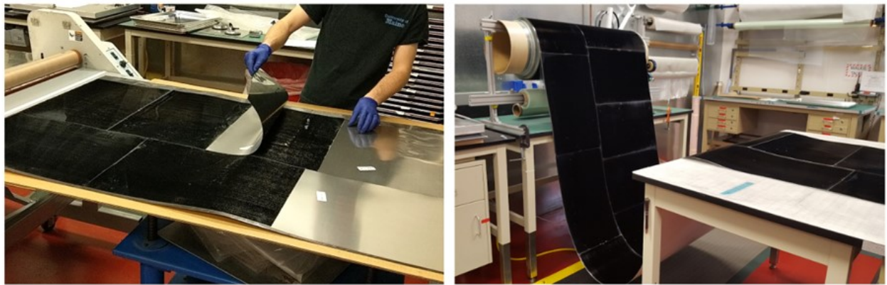
Figure 7. A photograph of transfer of the VACNTs into a roll of carbon fiber prepreg, and subsequent roll up of >100 \text{ m}^2 of the resulting NanoStitch® enhance prepreg for shipment to customers to fabricate and test full components.
