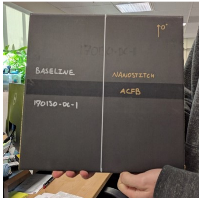
Figure 3. A standard composite panel fabricated with one half reinforced NanoStitch®, and the other side unmodified prepreg from the manufacturer.
