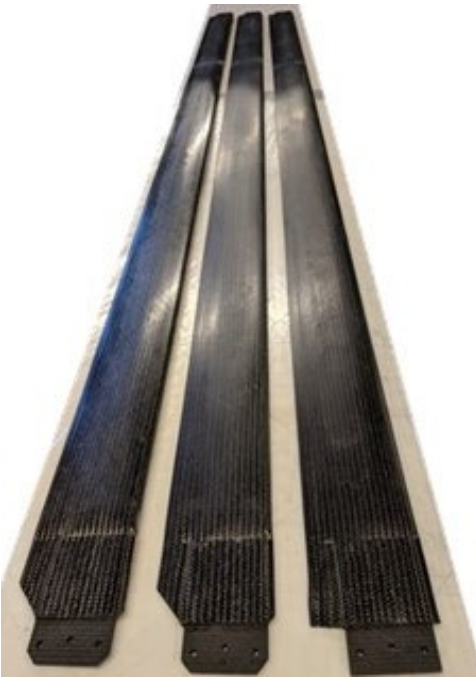
Figure 51: End-fitting Plates being fusion bonded to the Trimmed 129" blades
