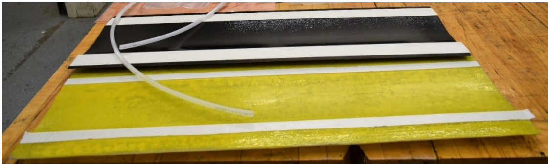
Figure 17: 32” molds manufactured from MDF master
