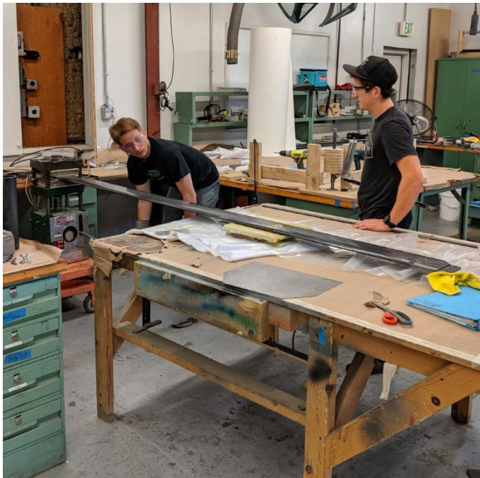
Figure 51: End-fitting Plates being fusion bonded to the Trimmed 129" blades
