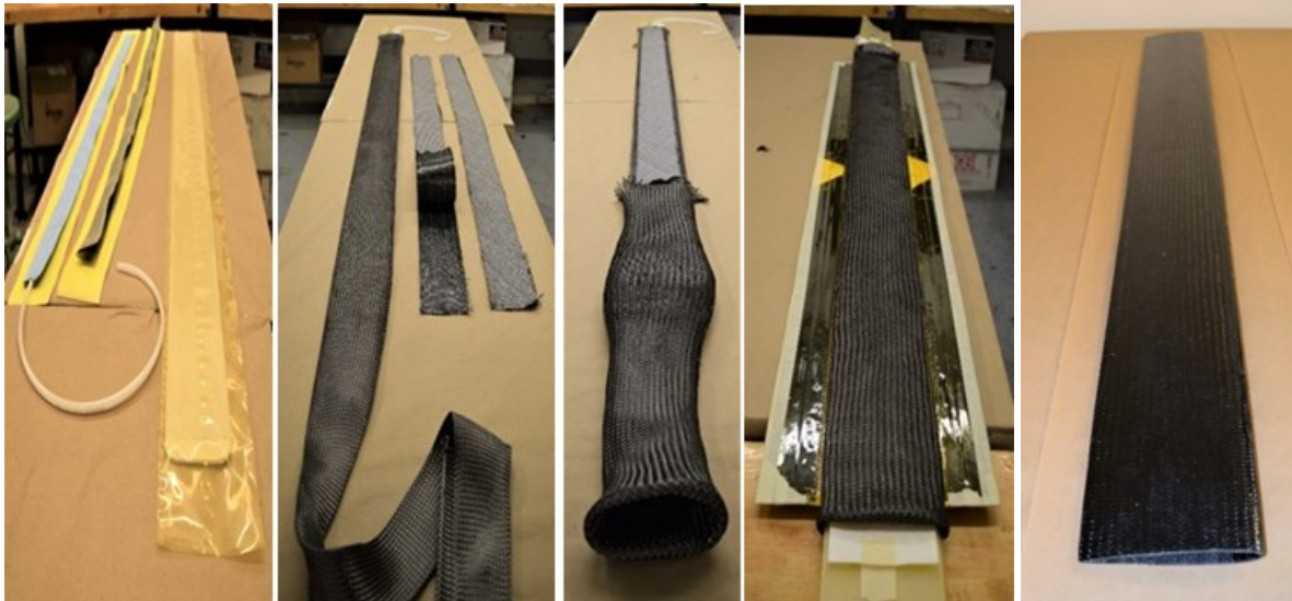
Figure 24: Adaption of 64" manufacturing process to braided carbon fiber. From left to right shows the consumables, preform set-up, placement of the final ply, preform in mold, and the 64" carbon fiber airfoil.
