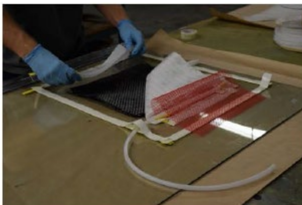
Figure 36: Flat plate trial infusion with Arkema Elium® 150 resin system
