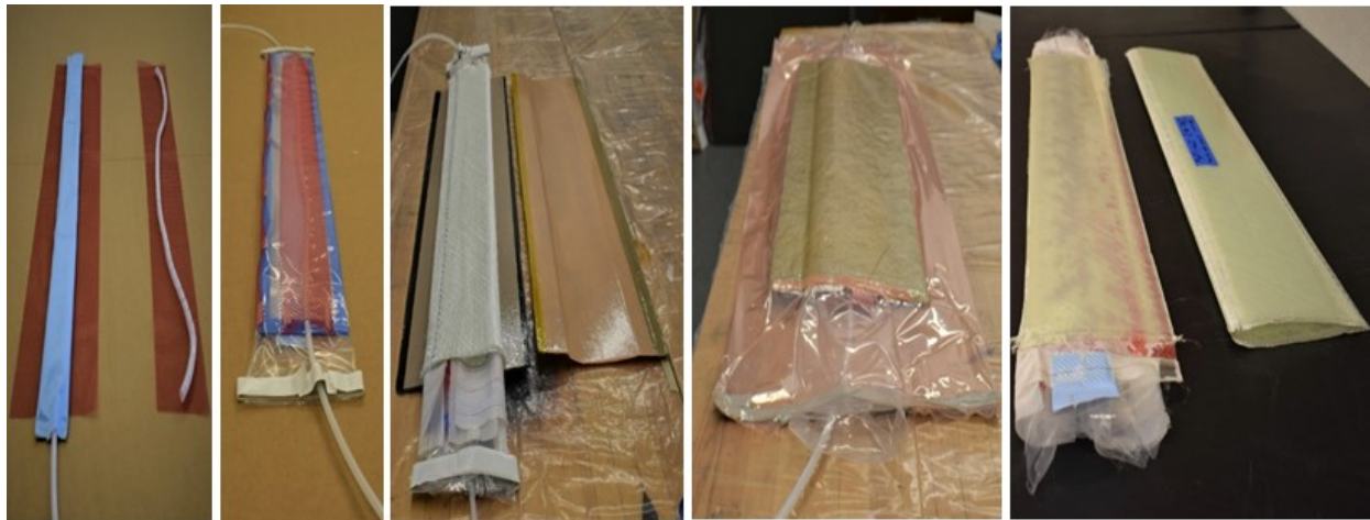
Figure 19: Initial manufacturing process to infuse a 32"-long hollow airfoil cross section. From left to right shows the Resin inlet and outlet, Consumables on the mandrel, preform in mold, fully bagged mold, airfoils after demolding.
