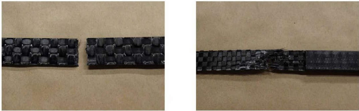
Figure 39: Representative failure modes of tensile specimens showing good cohesive failure at left with poor fiber interface pictured at right
