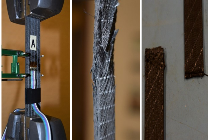
Figure 40: Examples of mechanical testing samples. In-plane shear modulus specimen with strain gages and clip-gage extensometer mounted (left), In-plane shear strength (middle), and Tensile strength (right)
