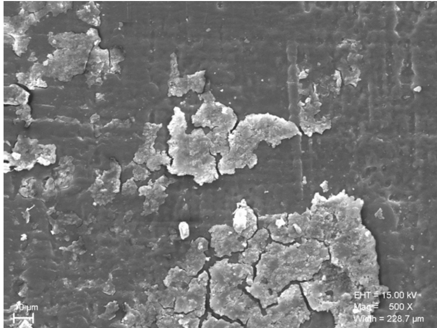
Figure 2. Debris on the surface of an “as cut” coupon, resin rich region.
