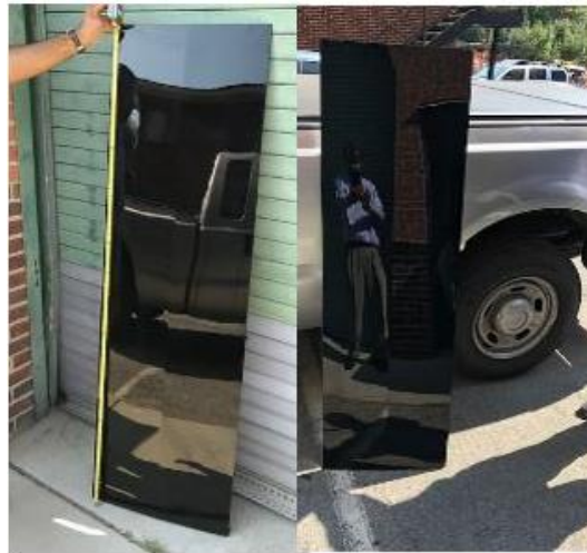
Figure 94. Painted and finished class-A SMC tractor hood part for demonstration
