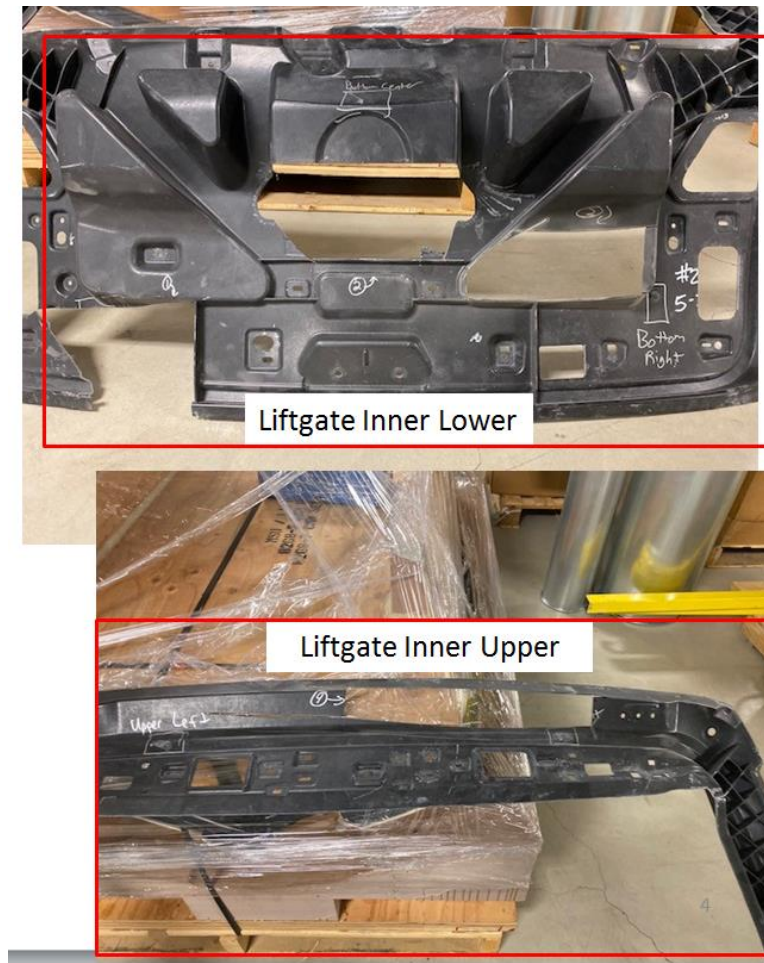
Figure 60. Example inner lift gate showing regions of interest for dynamic mechanical analysis (DMA).
