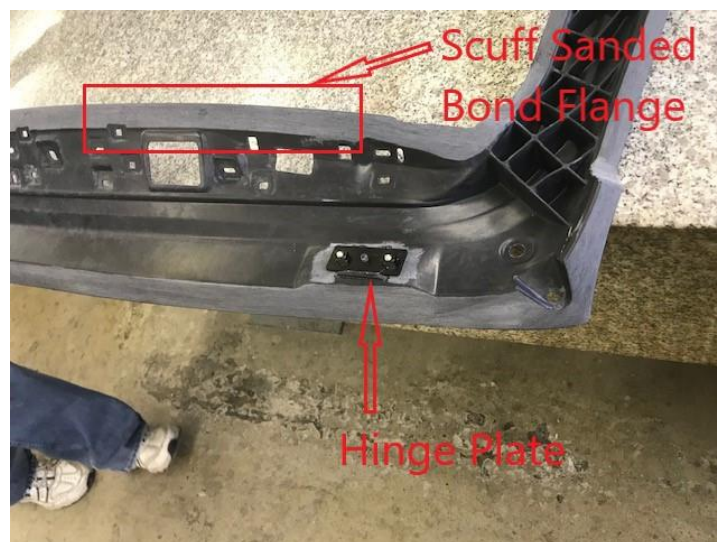
Figure 55. Denotes scuff sanded bond flange and placement of hinge plate reinforcement.
