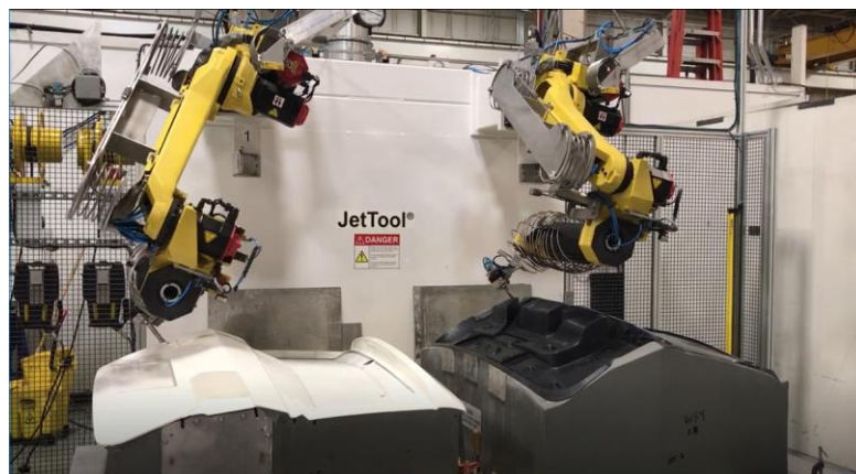
Figure 50. Trimming set-up at SPA for inner and outer panels.
