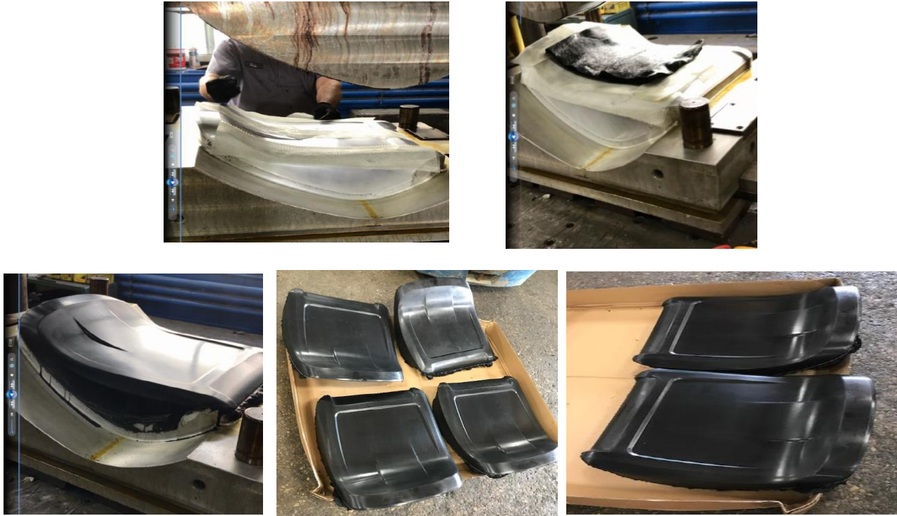
Figure 86. Illustration of parts molded under 300 s cycle time with M-211, one of the identified systems. (a) tape placement in the seat periphery and center; (b) SMC placement about 2/3 rd mold coverage; (c) example of molded SMC seat, still in the tool; (d) molded SMC seats for repeatability, and (e) molded seats with peripheral and center overmolded tape (on back side)
