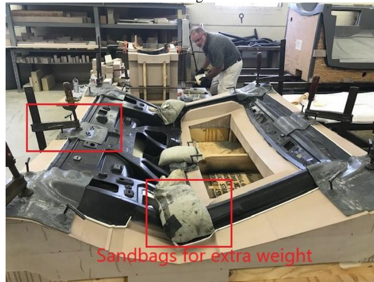
Figure 57. Denotes an assembly ready for bake cycle with clamps and sandbags to achieve adhesive contact.
