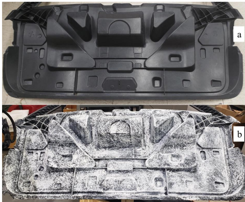
Figure 58. Images showing portion of liftgate (a) prior to and (b) after applying speckle pattern.
