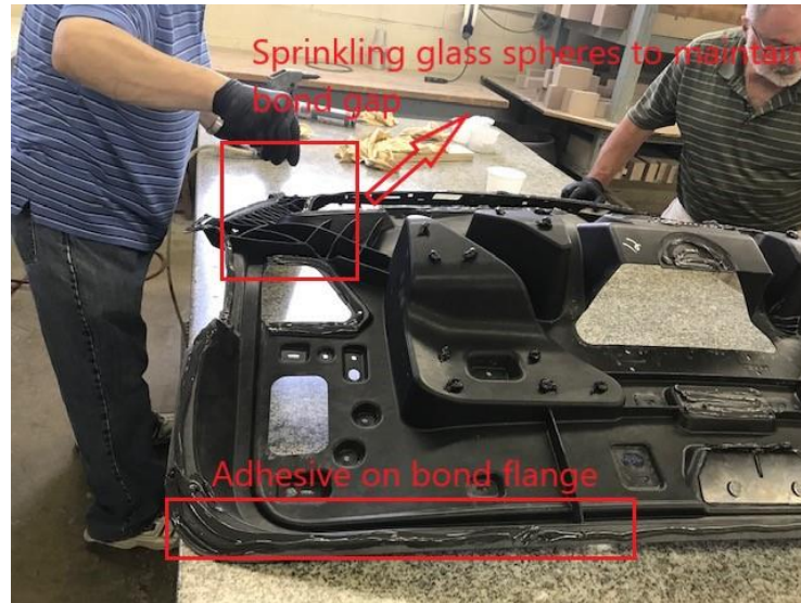
Figure 56. Highlights hand application of glass beads, mastic locations and applied adhesive to bond flange.
