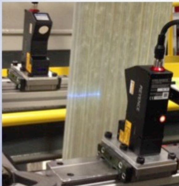
In-line diagnostics of tow form
