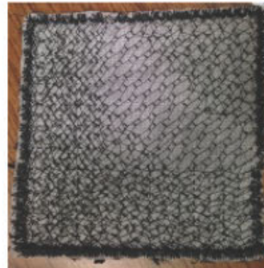
Back Side – Quasi-Isotropic Laystitch preform. Differential amount of stitching is an artifact of the number of layers printed to show the quasi-isotropic nature of the preform.
