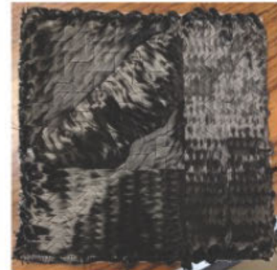
Front Side – Quasi-Isotropic Laystitch preform ( 0, +/- 45, 90 Degree Layers all visible).
