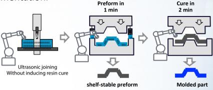
3. Automated fast ply cutting, lay-up, preforming & molding
