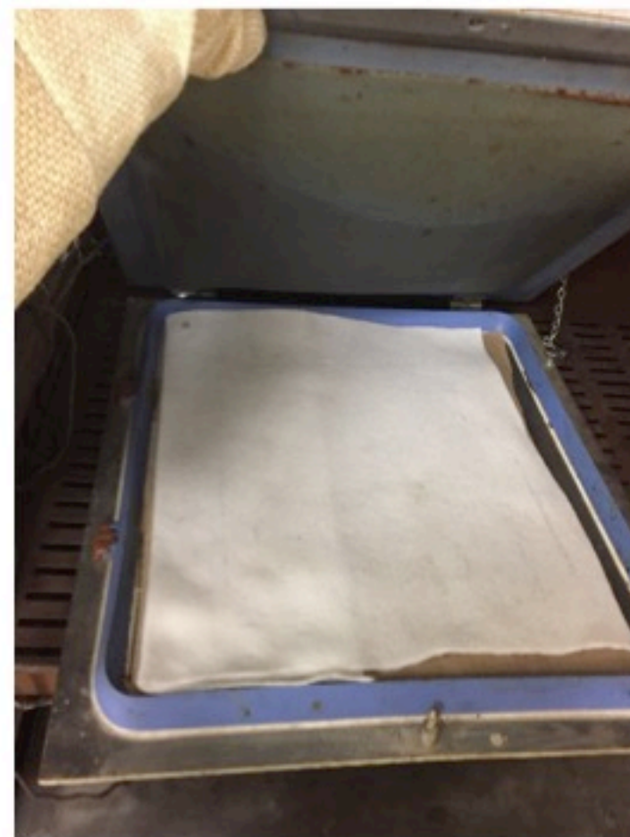
Compression Molding at 325 – 350°F, 100 psi, 3 min
